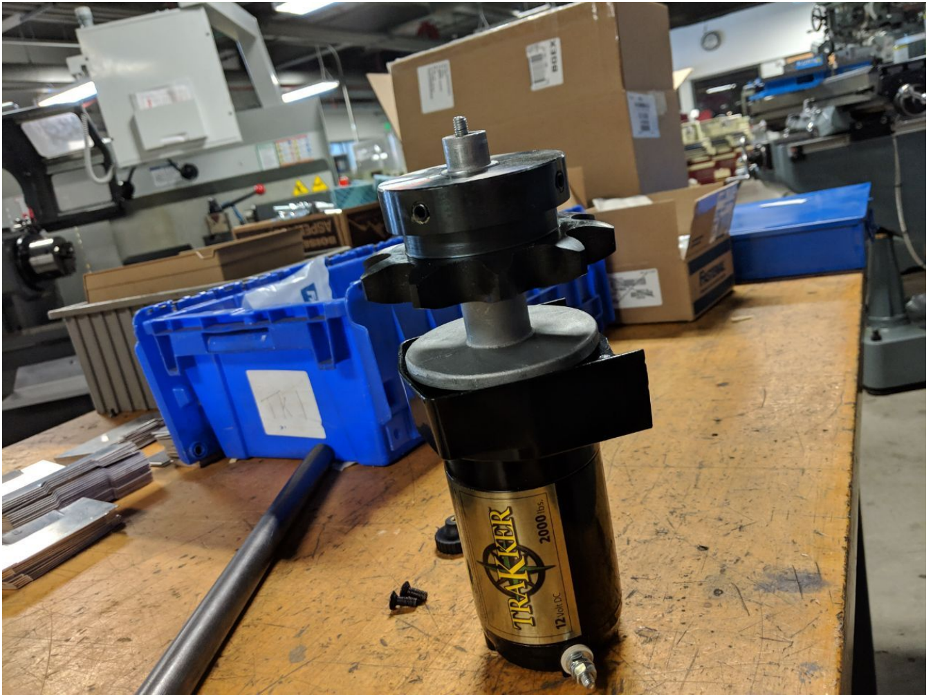
Photo of fitting the sprocket to the freshly turned outside diameter of the winch spool
