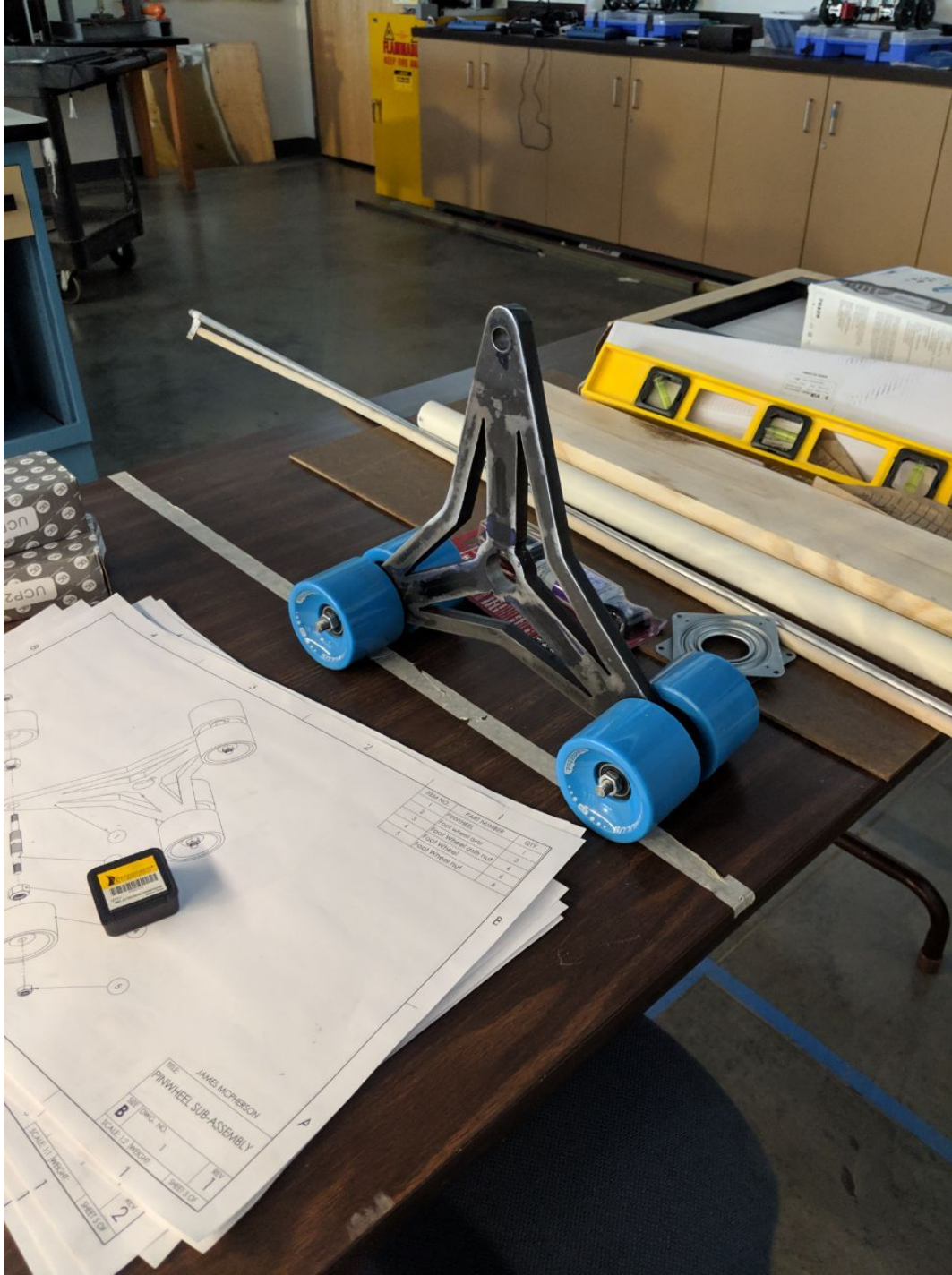
Photo of partially finished pinwheel. This is the Pinwheel that turned out nicer. The other pinwheel got chewed up pretty badly by the plasma cutter
