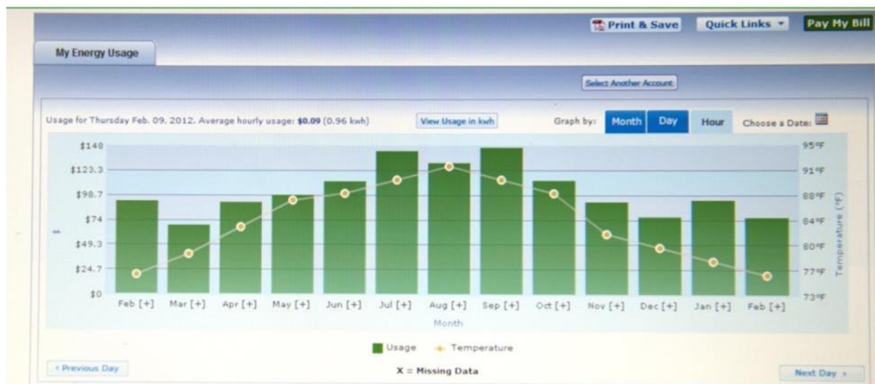
Figure 12. EMIS Smart Meter Web Page. Source: Florida Power & Light (2016).
