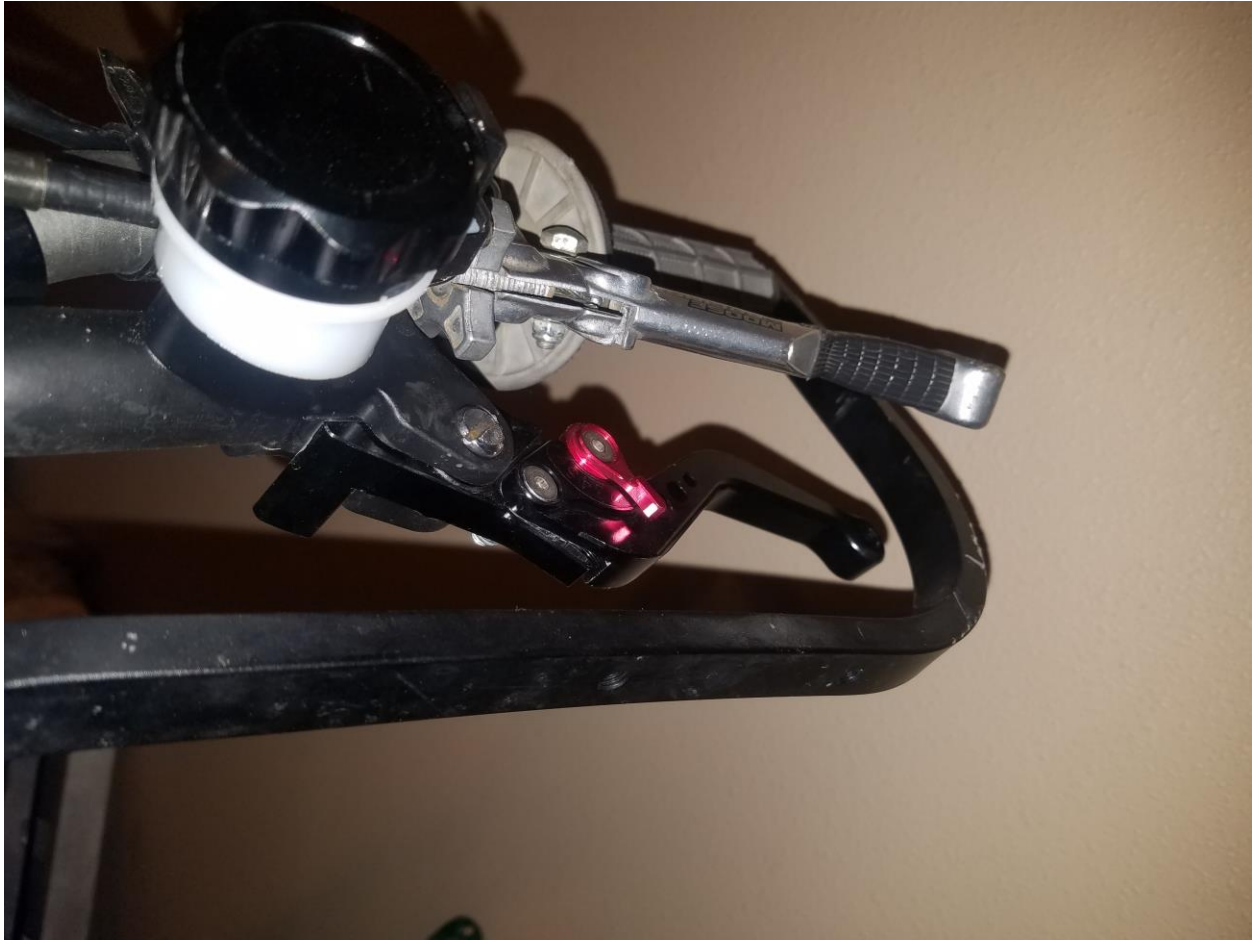
Figure 20, Lever set up. Upper lever (silver/black) is for the clutch Lower lever (black/red) is for rear brake
