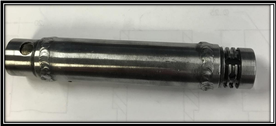
L4: Welded Adapter/Adapter Tube and Ball Nut
