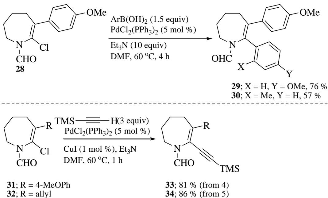
**Figure 1-22** Palladium-catalyzed  $\alpha$ -arylation and alkylation of C2-functionalized cyclic  $\alpha$ -chloro eneforamides
