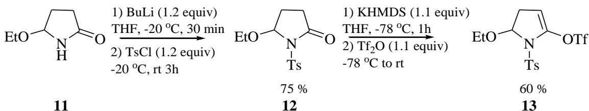
**Figure 1-16** Preparation of vinyl triflates from an ethoxy lactam
