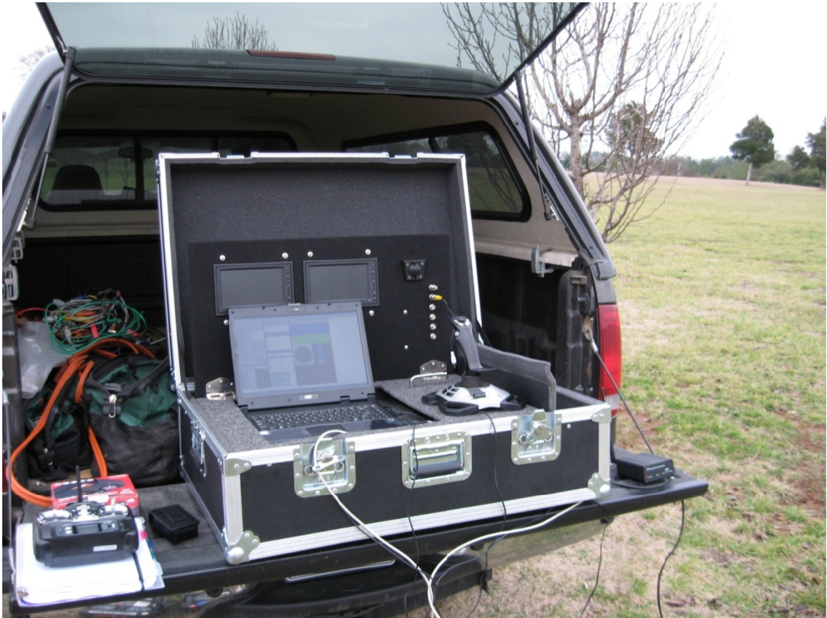
Figure 5-3. The ground control station for semi-autonomous and full-autonomous flight control of the aerial surveillance vehicle.
