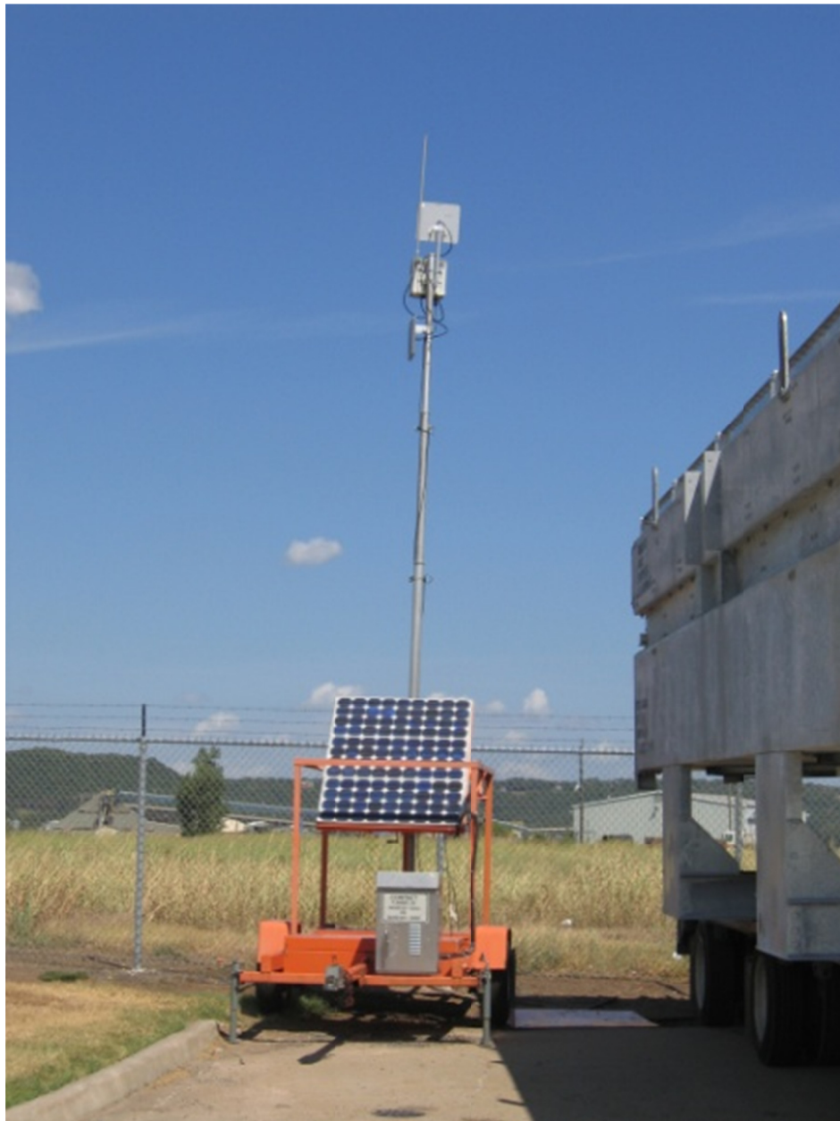
Figure 9-2. STRIX™ wireless network node mounted on ODOT provided trailer.
