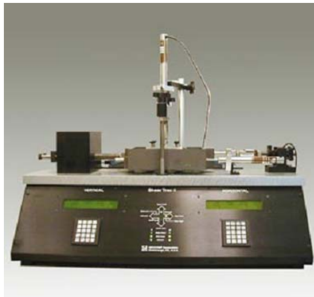
Figure 3.3: Unmodified Direct Shear Device
