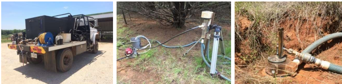
Figure 2.3. Controlled-burn truck used to provide water to field site (left), head tank that delivers constant pressure to JET and recycle loop to send water back to tank (middle), and JET device in field (right).
