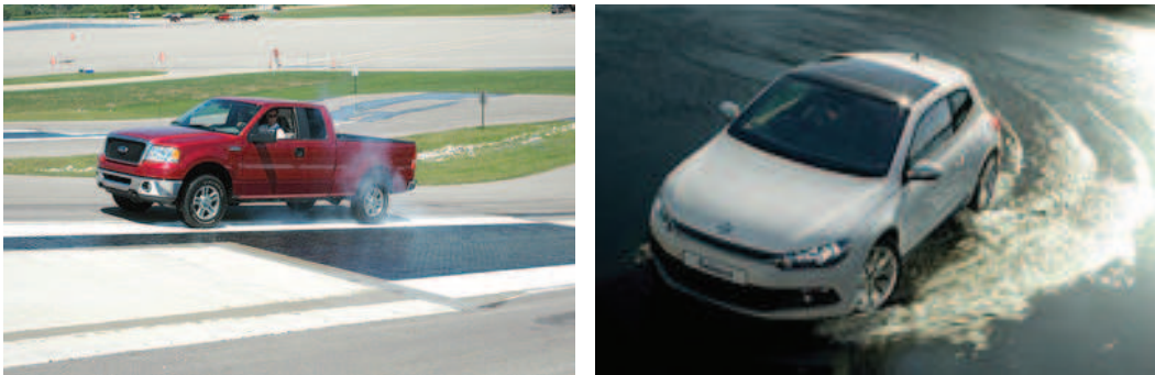
Figure I.2: Longitudinal [7] and lateral slip [8]
