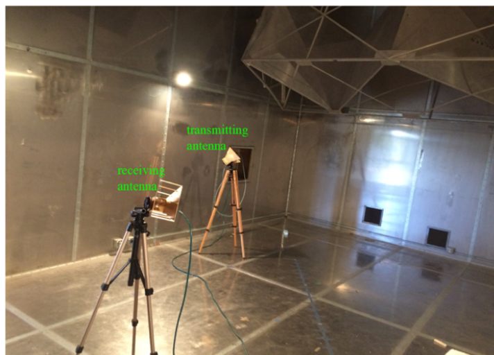
Figure 6.5. Quality factor measurement using two dual-ridged horn antennas
