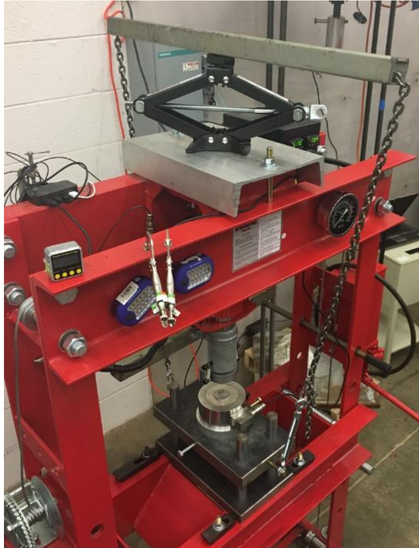
Figure 5.13: Chains attaching top plate to scissor jack
