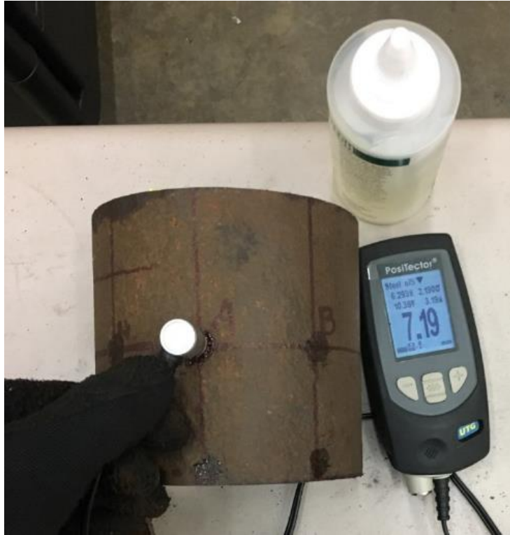
Figure 5.17: Using Positector ultrasonic tool to measure wall thickness
