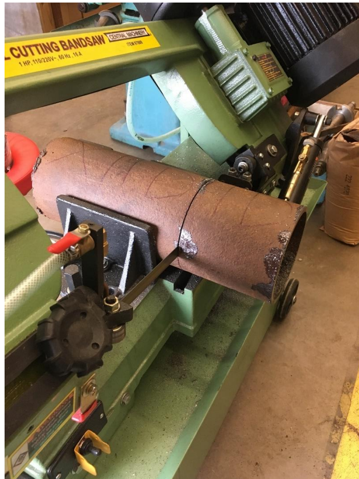
Figure 5.14: Band saw cutting pipe
