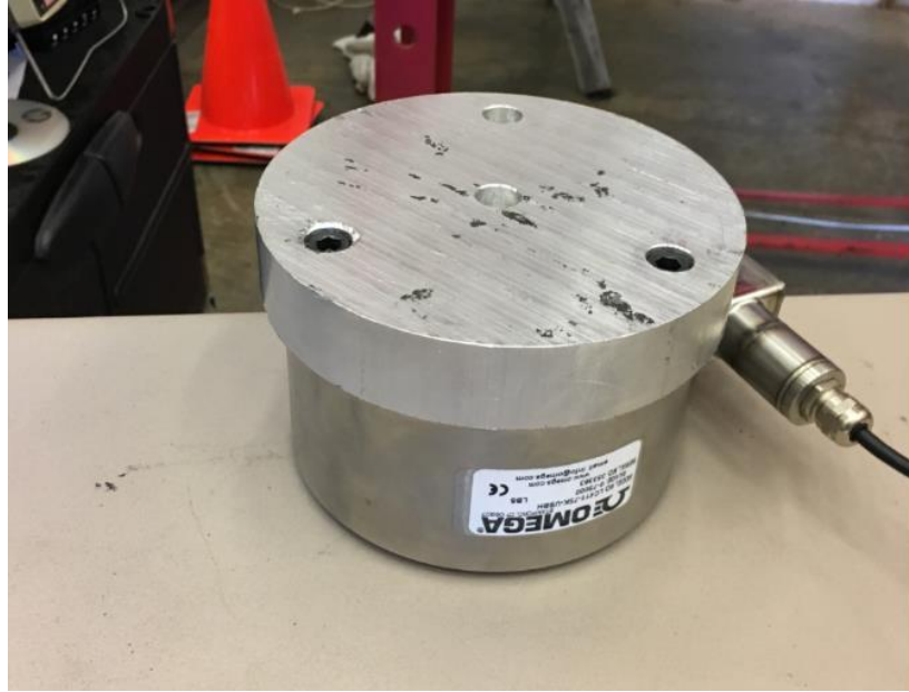
Figure 5.7: Omega force gauge bolted to aluminum plate
