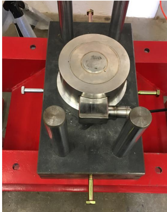
Figure 5.9: Holes drilled in hydraulic press
