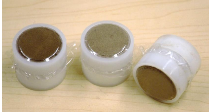
Figure 2.3: Packed circular XRF soil sample cups lined with polypropylene X-ray film for analysis
