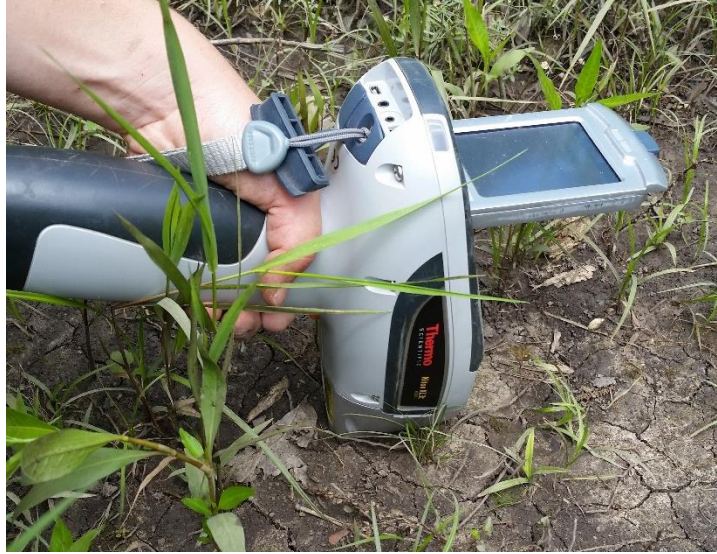
Figure 2.2: The field portable Thermo-Fisher Scientific Niton XL3t GOLDD+ XRFs being operated in situ on a soil surface with all debris removed
