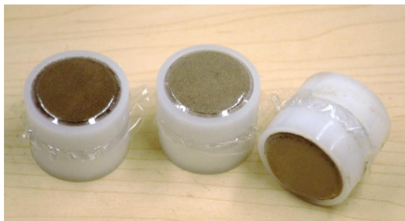
Figure 3.5: Packed circular XRF soil sample cups lined with polypropylene X-ray film for analysis
