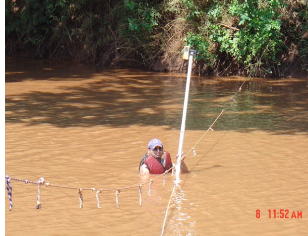
Figures 4.4 Survey of channel cross-section in Skeleton Creek
