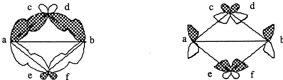
Figure 11. Bonding and Antibonding Molecular Orbitals Formed from Combinaton of Two p_y Orbitals of Copper atoms and two sp^3 Orbitals of Iodide Atoms
