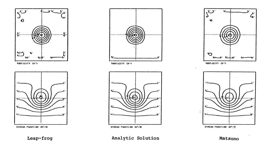
Fig. 13. Comparison of Leap-frog and Matsuno time differencing with consistent mass after 120 hours using the 4-node finite element for the vorticity-stream function model.
