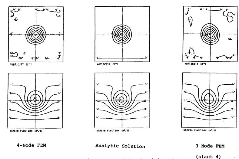
Fig. 7. Comparison of 4-and 3-node finite elements with Crank-Nicholson time difference and consistent mass after 120 hours for the vorticity-stream function model.
