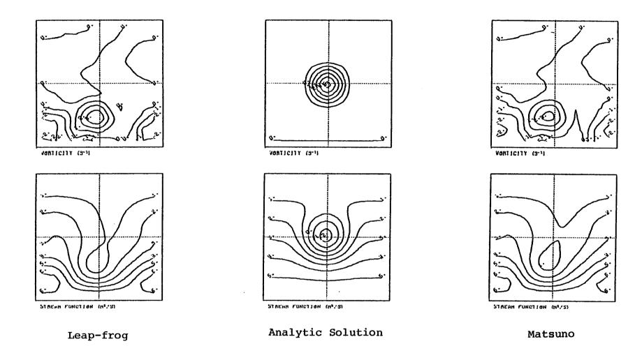
Fig. 15. Comparison of Leap-frog and Matsuno time differencing with lumped mass after 120 hours using the 4-node finite element for the vorticity-stream function model.
