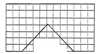
Fig. Al. Discretization of domain for finite differences.
