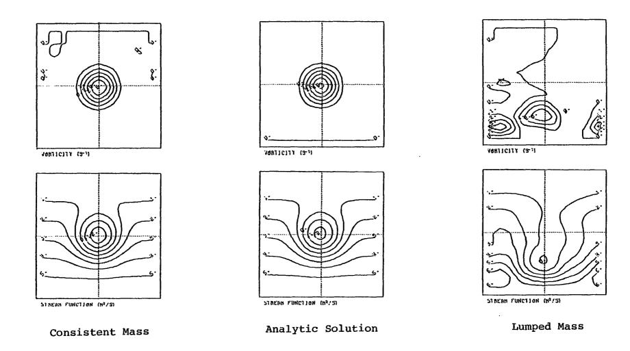
Fig. 17. Leap-frog time difference with Arakawa Jacobian finite difference in space. (vorticity-stream function model)
