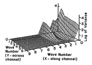
Fig. 6. Fourier analysis of initial height field for shallow water equations
