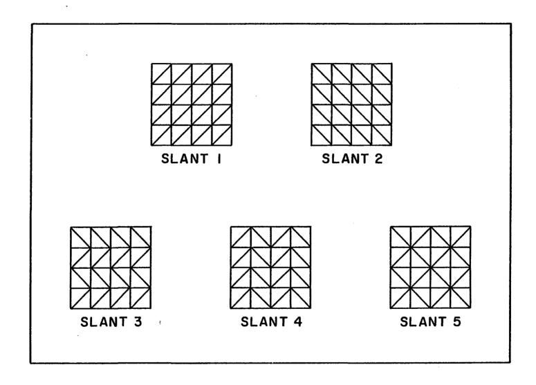
Fig. 5. Arrangement of triangular elements within the mesh
