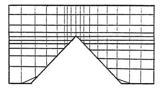
Fig. A2. Discretization of domain for finite element method.
