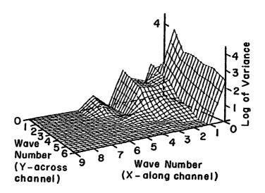
Fig. 25. 48 hour forecast height field and Fourier analysis from shallow water equations using Leap-frog time differencing.
