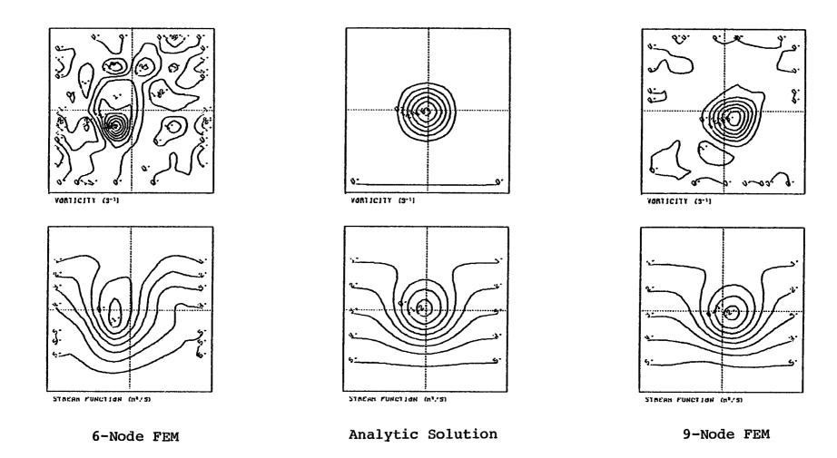
Fig. 12. Comparison of 6-node and 9-node finite elements with Crank-Nicholson time difference and lumped mass after 120 hours for the vorticity-stream function model.
