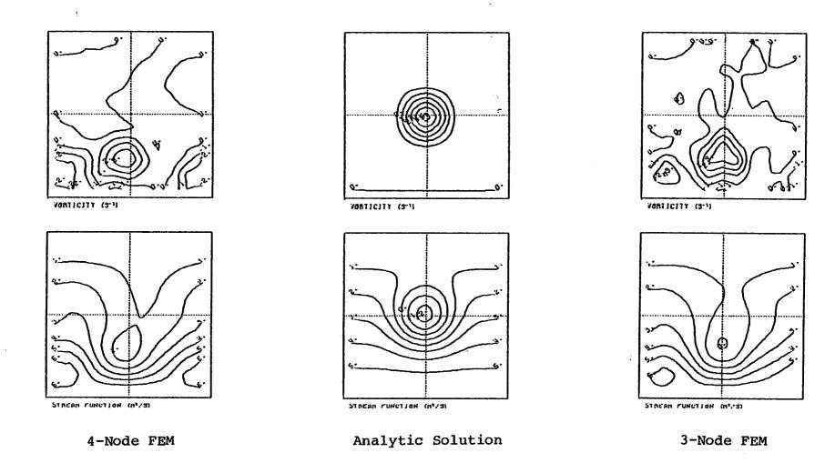
Fig. 11. Comparison of 4-node and 3-node finite elements with Crank-Nicholson time difference and lumped mass after 120 hours for the vorticity stream function model.
