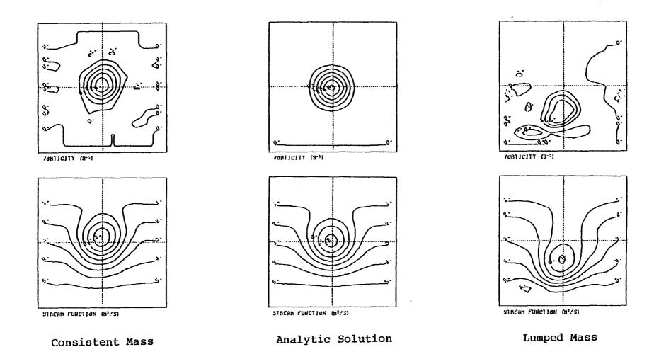
Fig. 18. Leap-frog time difference with centered finite difference in space. (vorticity-stream function model)
