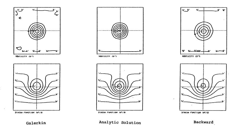
Fig. 14. Comparison of Galerkin and Backward time difference with consistent mass after 120 hours using the 4-node bilinear finite element for the vorticity-stream function model.
