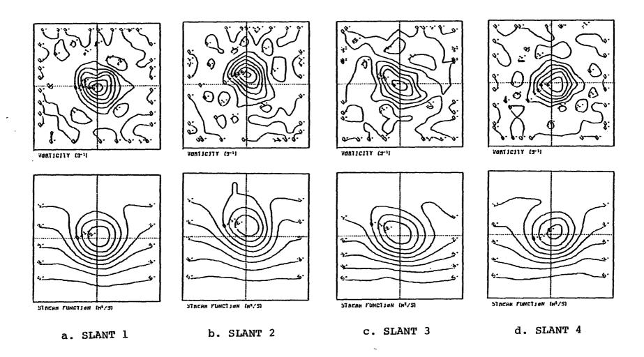
Fig. 10. 120 hour forecast of stream function and vorticity for four different arrangements of 6-node quadratic triangular element.
