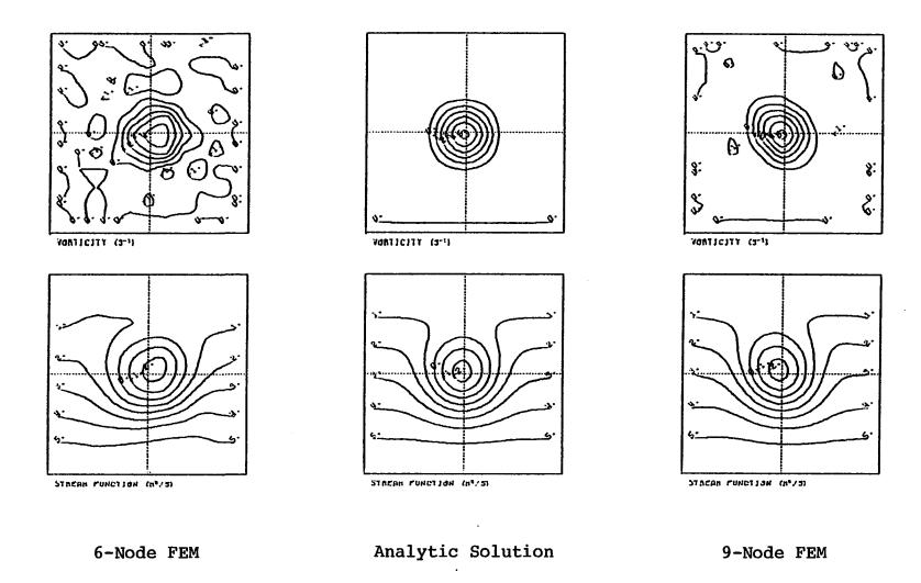
Fig. 8. Comparison of 6-and 9-node finite elements with Crank-Nicholson time difference and consistent mass after 120 hours for the vorticity-stream function model.
