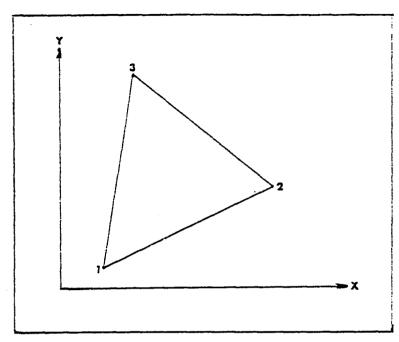
Fig. A3. Typical triangular element.
