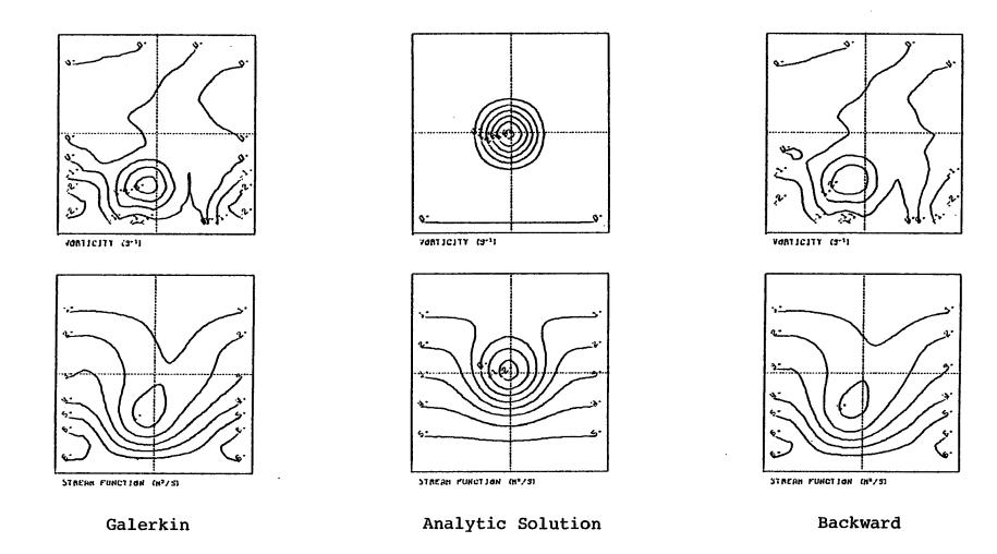
Fig. 16. Comparison of Galerkin and Backward time differencing with lumped mass after 120 hours using the 4-node finite element for the vorticity-stream function model.
