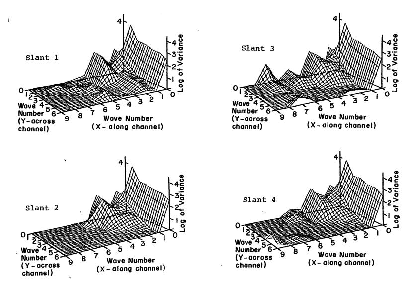
Fig. 23. Fourier analyses of 48 hour forecast height fields for four different arrangements of the linear triangular element.
