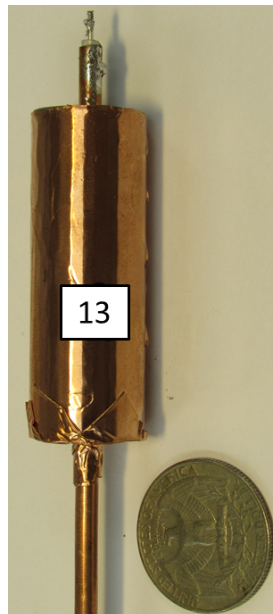
FIGURE 6.2: The final printed core dielectrically loaded unfolded balun with a standard American 25c coin for reference.
