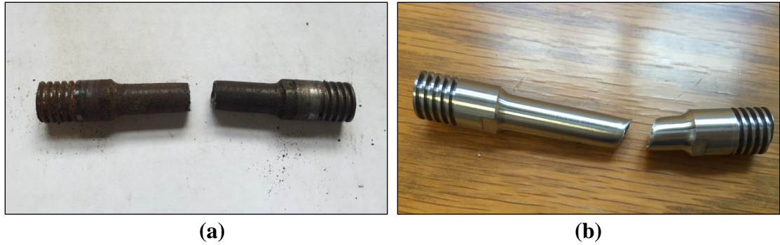
Figure 4.19: Comparison of features of brittle and ductile failures: a) Q-125-5; and b) Q-125-1 (baseline)
