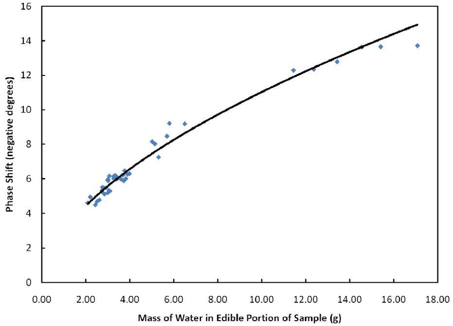
Figure 4.13: Edible kernel water vs. signal phase shift at 433 MHz
