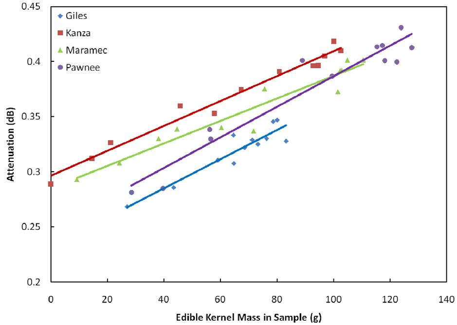
Figure 4.3: Edible kernel mass vs. signal attenuation at 408 MHz
