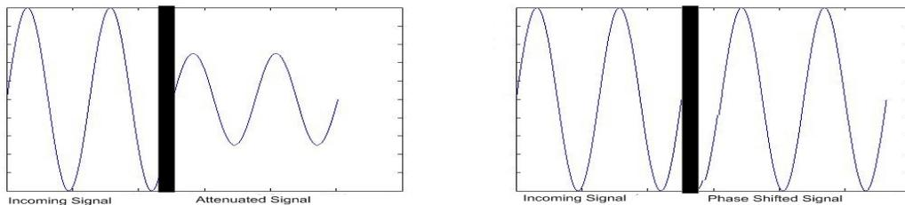
Figure 2.1: Attenuation and phase shift of a propagating wave
