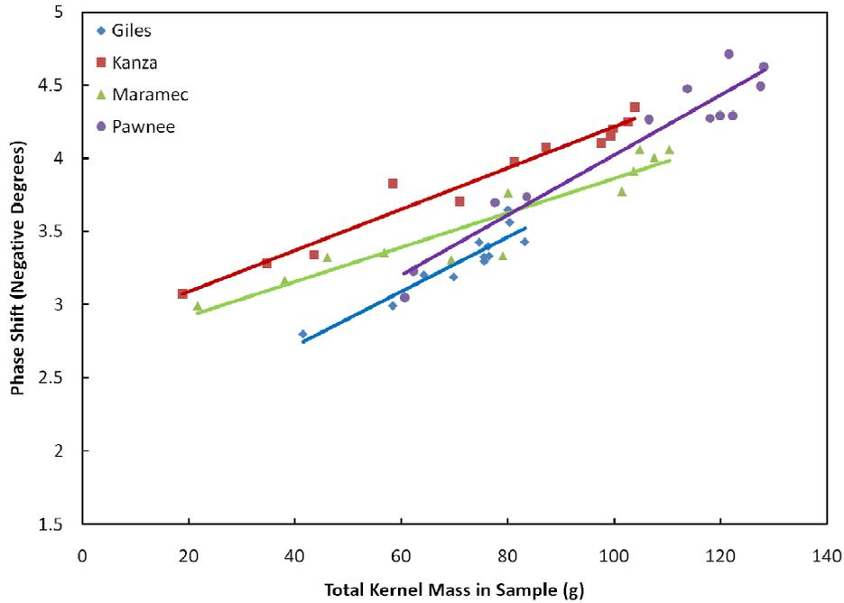
Figure 4.10: Total kernel mass vs. signal phase shift at 458 MHz
