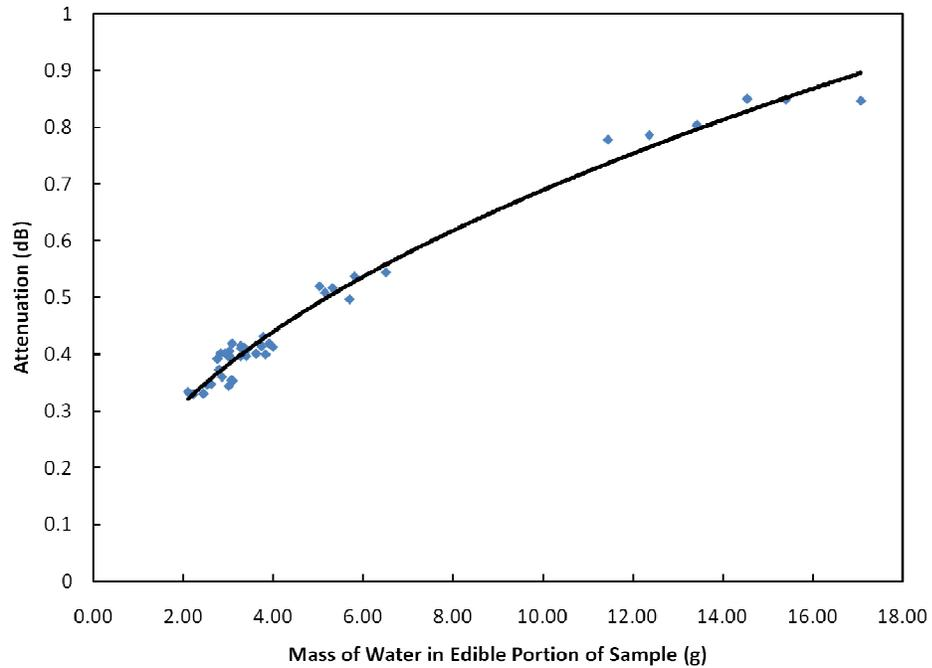
Figure 4.11: Edible kernel water mass vs. signal attenuation at 408 MHz
