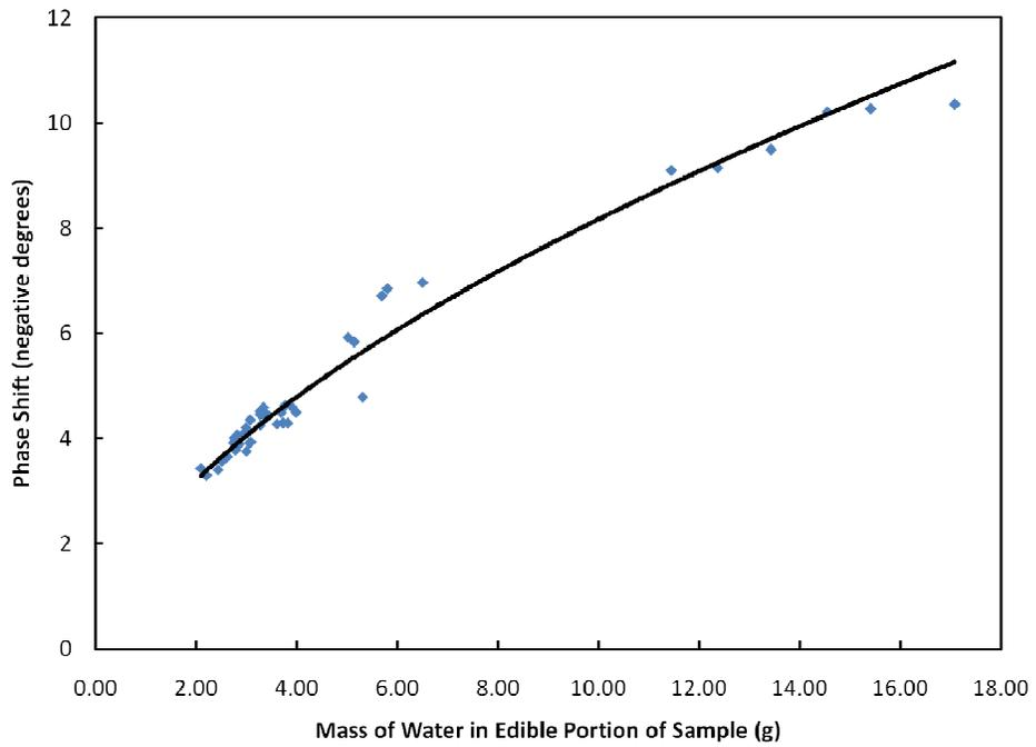
Figure 4.14: Edible kernel water vs. signal phase shift at 458 MHz
