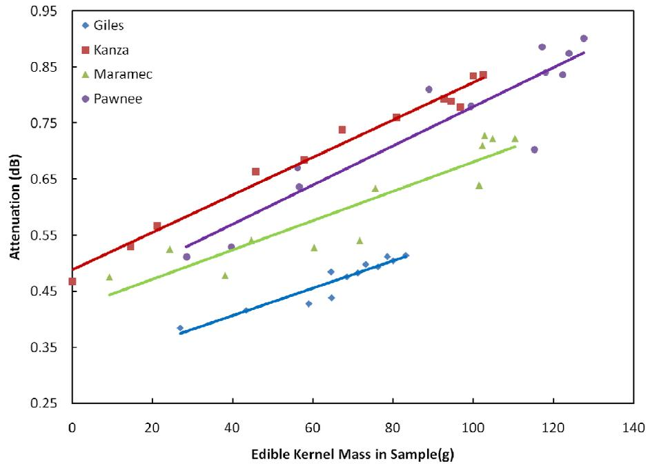
Figure 4.4: Edible kernel mass vs. signal attenuation at 1.03 GHz
