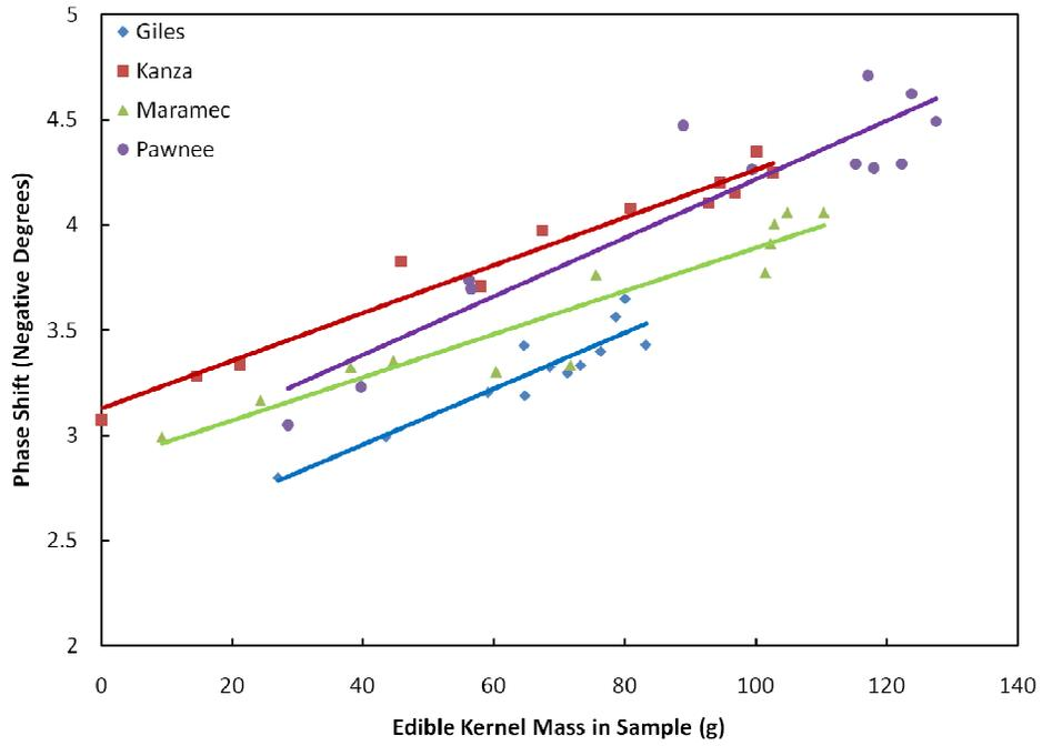
Figure 4.8: Edible kernel mass vs. signal phase shift at 458 MHz
