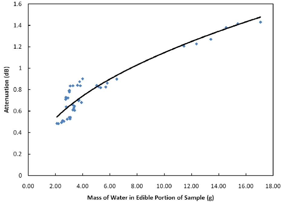
Figure 4.12: Edible kernel water mass vs. signal attenuation at 1.03 GHz
