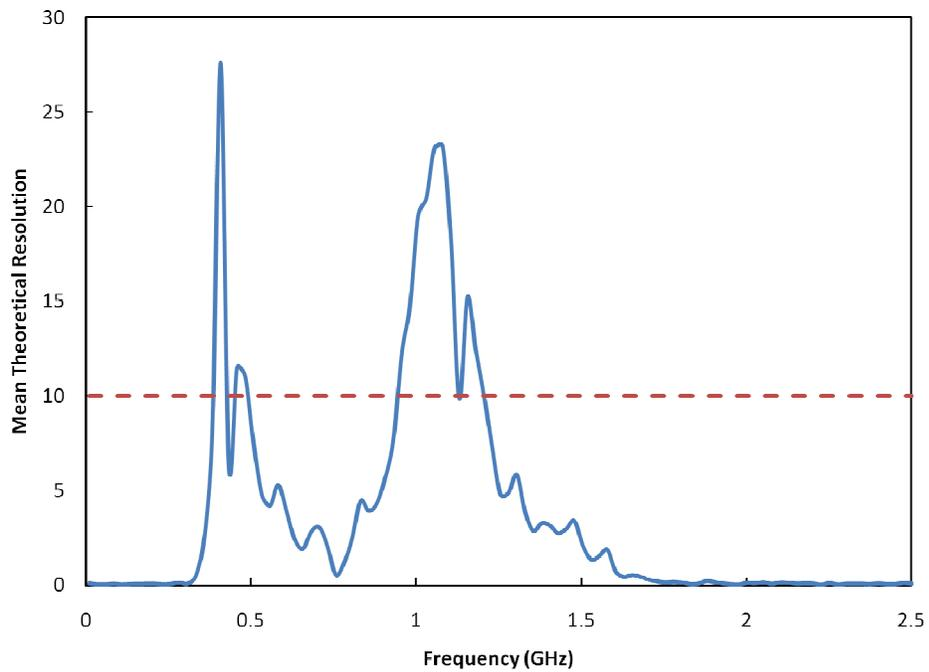
Figure 4.1: Mean theoretical resolution vs. frequency for signal attenuation with the threshold resolution value set at 10
