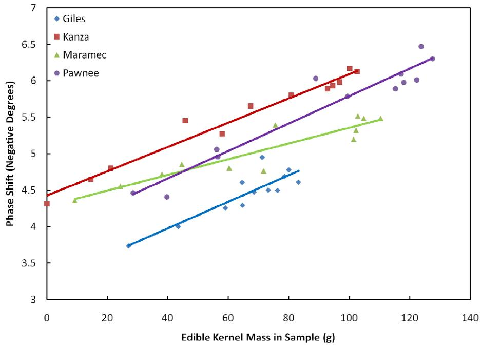
Figure 4.7: Edible kernel mass vs. signal phase shift at 433 MHz
