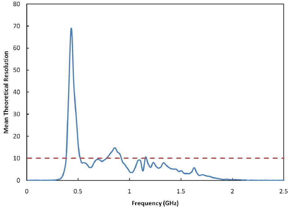
Figure 4.2: Mean theoretical resolution vs. frequency for signal phase shift with the threshold resolution value set at 10
