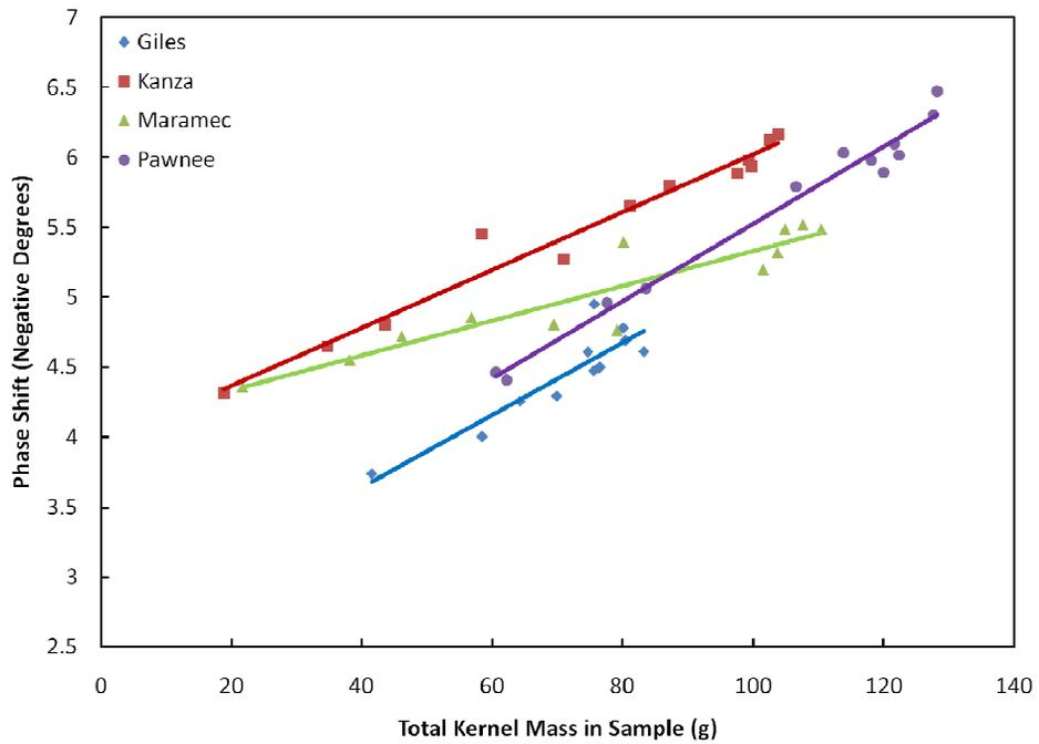
Figure 4.9: Total kernel mass vs. signal phase shift at 433 MHz
