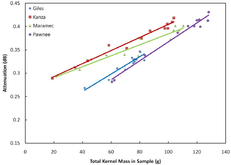
Figure 4.5: Total kernel mass vs. signal attenuation at 408 MHz
