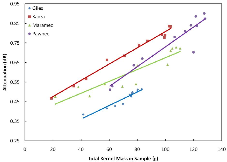
Figure 4.6: Total kernel mass vs. signal attenuation at 1.03 GHz
