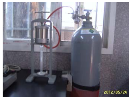
Figure 4 Measurement apparatus for fluid loss properties
