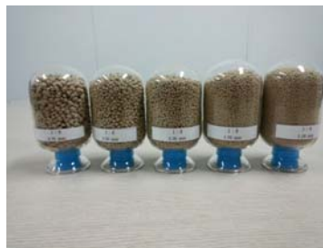
Figure 2 Mixed grout granules of bentonites and sands
