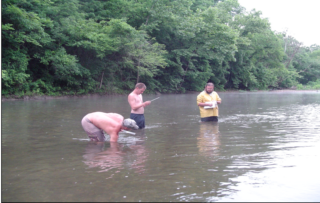
Fig. 5.3. Mark Murphy, Raymond Ary, and Kyle Winters measuring the A, B, and C axes of particles on Spavinaw Creek in the Ozark Highlands. Survey date was June 6, 2004.
