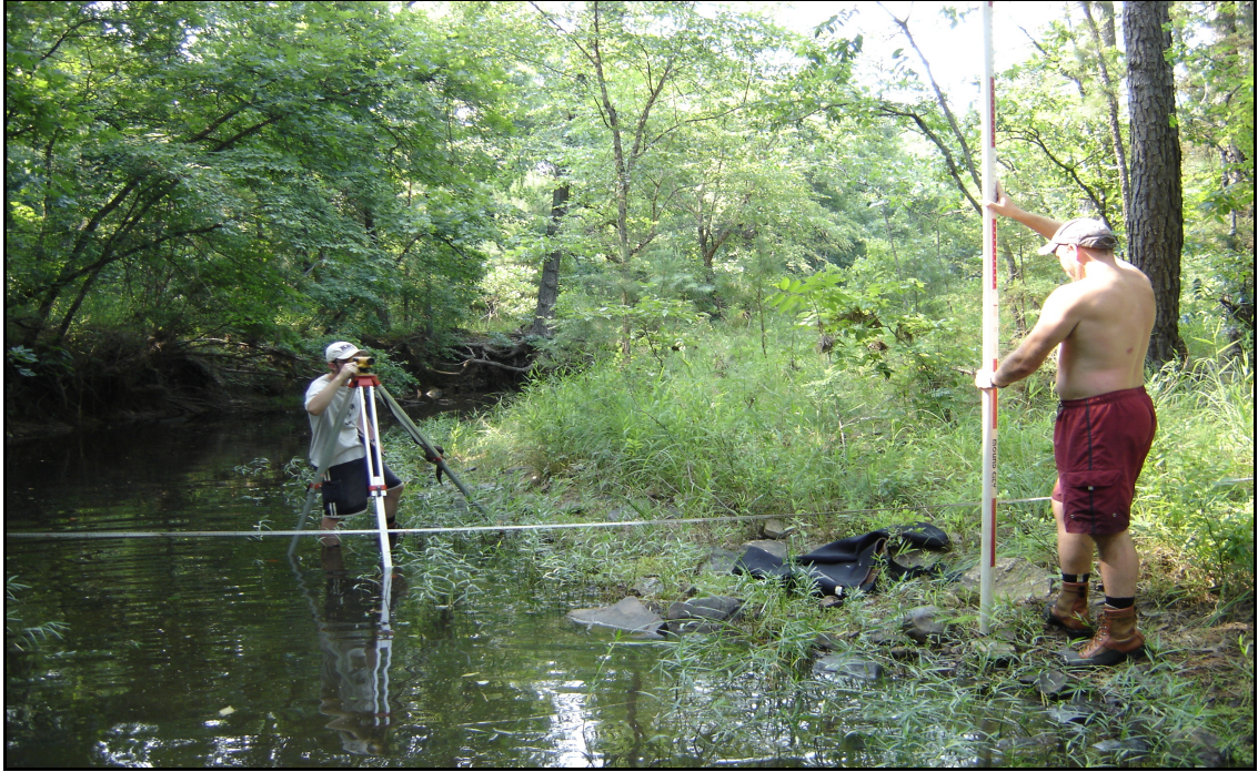
Fig. 3.2. Bryce Marston (tripod and level) and Dale Splinter (stadia rod) conducting a cross-sectional survey of a stream in the Ouachita Mountains ecoregion.
