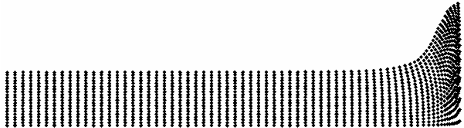
Figure 39. Deformed shape represented by material points at 24 \mu\text{s}
