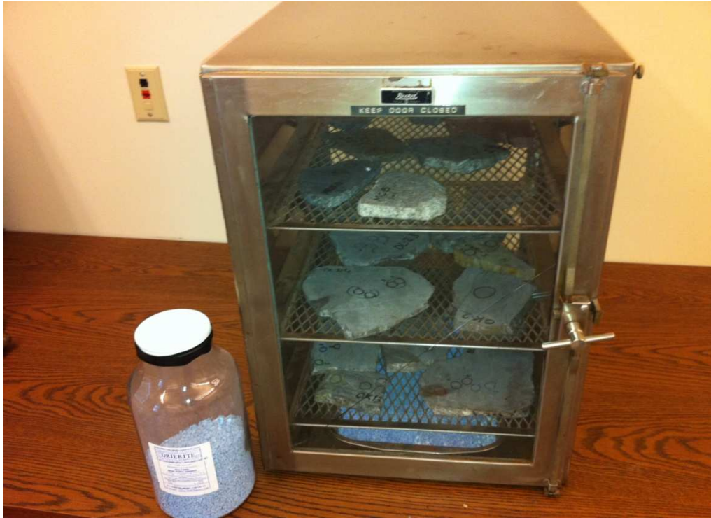
Figure 4-6 The desiccator with anhydrous calcium sulfate crystals
