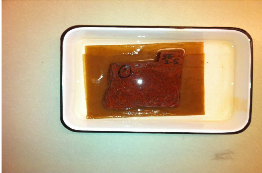
Figure 4-5 Cleaning the sample with hexane
