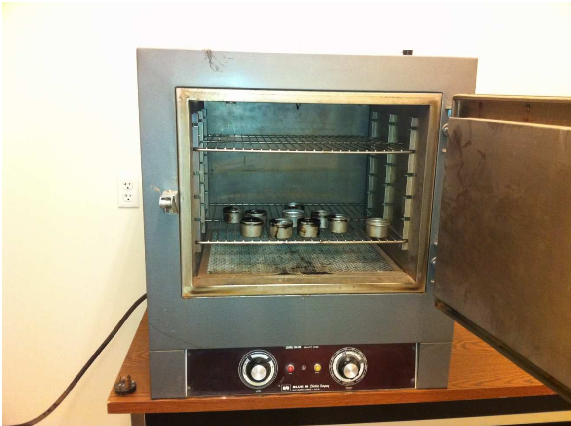
Figure 4-11 PG 64-22 Binder divided into a number of tin canisters and kept in the oven
