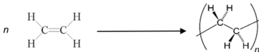
Figure 1 Polymerization of ethylene into polyethylene
