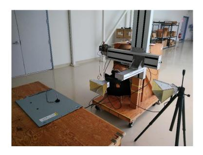
Figure 3.2: Typical ESM test configuration. In this photo, debugging data processing system of the ESM.
