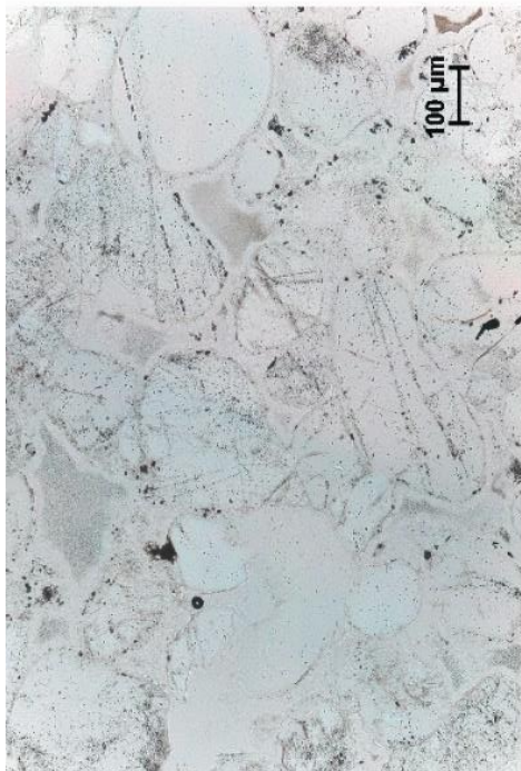
Figure 37. Comparison of 5GN1 and Parlin Flats with differential thickness in the chalcedony cement. Notice the intrusions in the Parlin Flats quartz grain in the center right. Both are taken at 10X with plane and cross-polarized top and bottom respectively.
