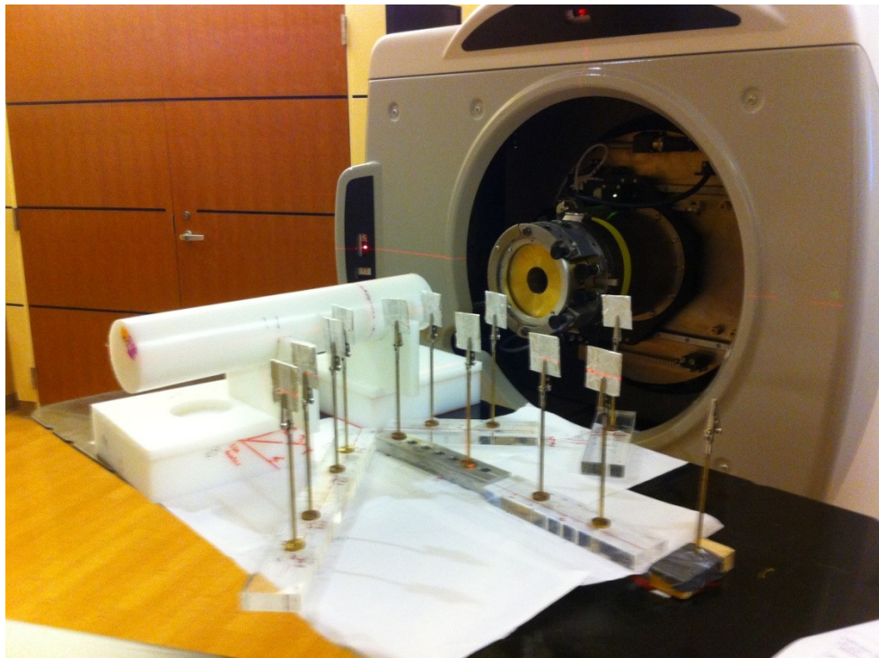
Figure 5.7: Diagram of the cylindrical-phantom experimental setup where filled circles represent the detectors locations (top), picture taken during the actual experiment (bottom).
