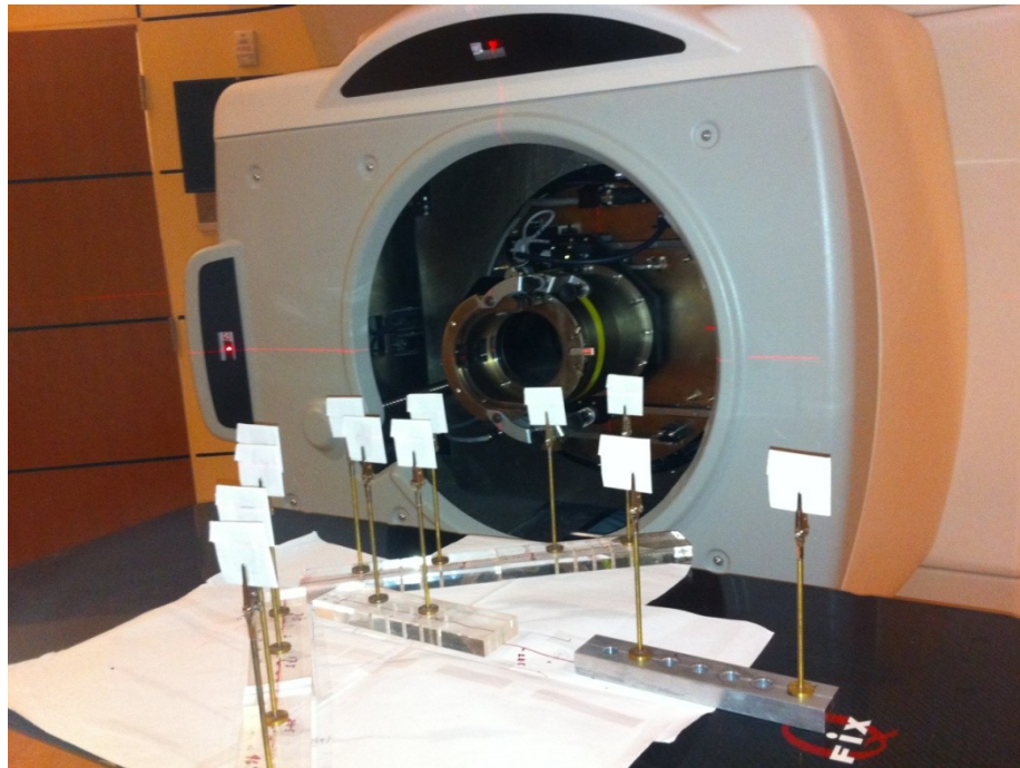
Figure 5.5: Diagram of the in-air experimental setup. Circles represent the detectors locations in the air. Picture was taken during the actual experiment (bottom).
