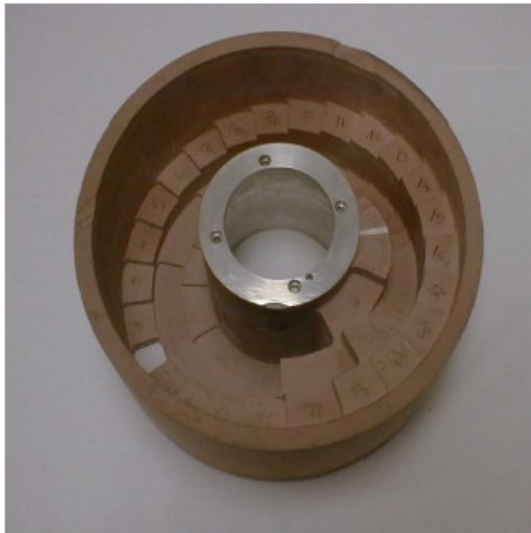
Figure 2.6: A common range modulator wheel used in proton radiotherapy. Picture taken from (Schlegel et al., 2006).
