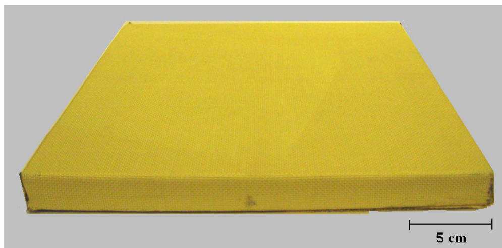
Figure 13 Perspective side view of the Composite plate with Kevlar wrap.
