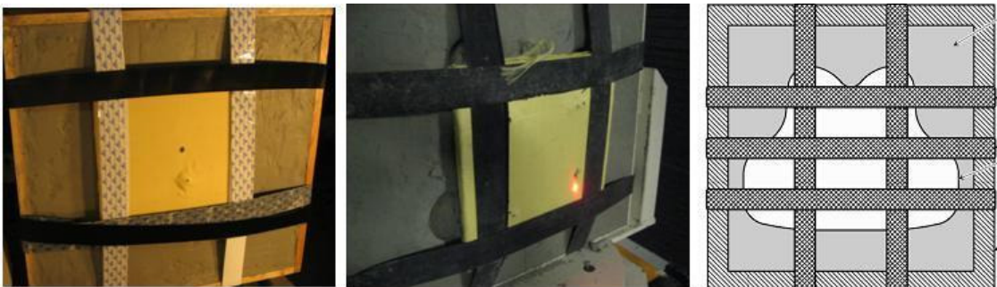
Figure 15 Mounting of plates on clay backing using Velcro straps.
