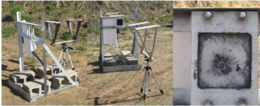
Figure 16 Perspectives of Rigid steel frame setup to test 4130 plates with front and back chronograph.
