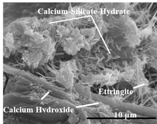
Figure 12: Ettringite (white, needle-like crystals) are commonly found in samples taken from concrete in service
