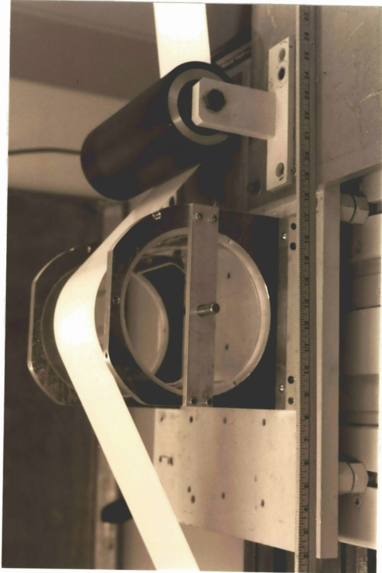
Figure 21. Modified Test Set-Up for High Wrap Angle ( \beta=60^\circ )
