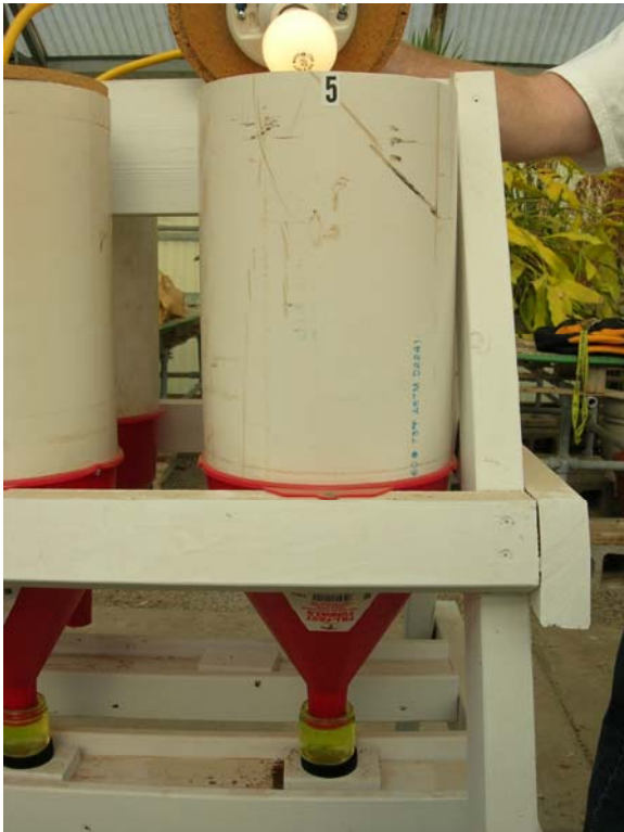
Figure 2.1. Berlese funnel used to remove aphids from wheat seedlings
