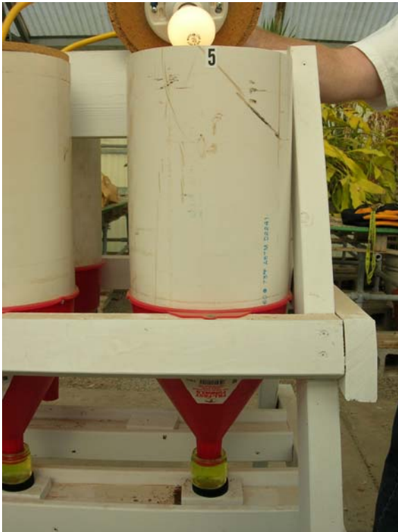
Figure 5.1. Berlese funnel used to remove aphids from wheat seedlings
