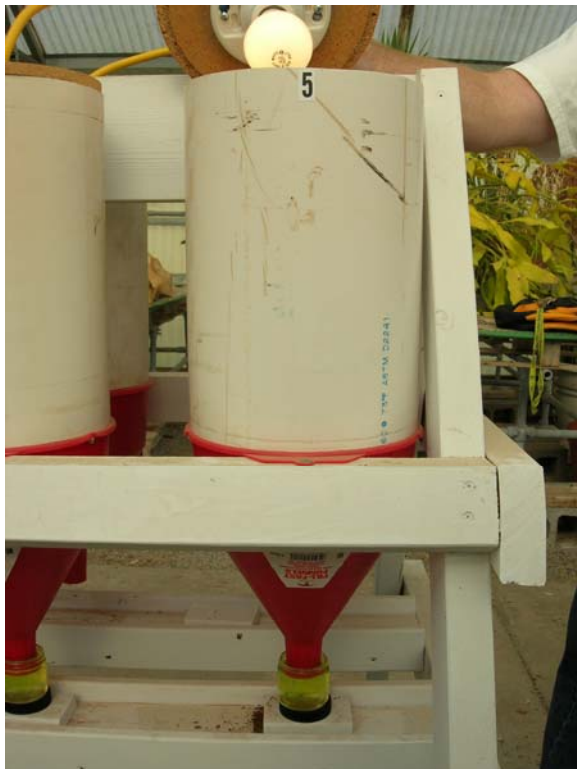
Figure 3.1. Berlese funnel used to remove aphids from wheat seedlings
