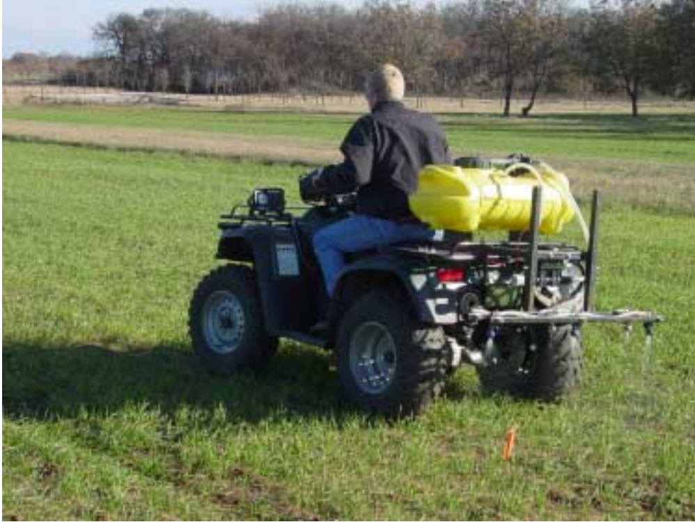
Figure 4. Applicator used to apply Nitrogen Calibration Strips in 2004-5005.
