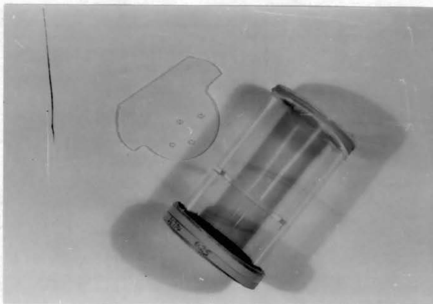
Fig. 12.--Test cylinder, shutoff slide, slot, cheese cloth cover, and treated membrane.
