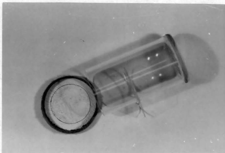
Fig. 13.--Test chamber with shutoff slide assembled and membrane treated area marked.
