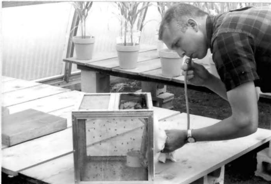
Fig. 2.--Stillwater stable fly cage and mouth operated aspirator tube.
