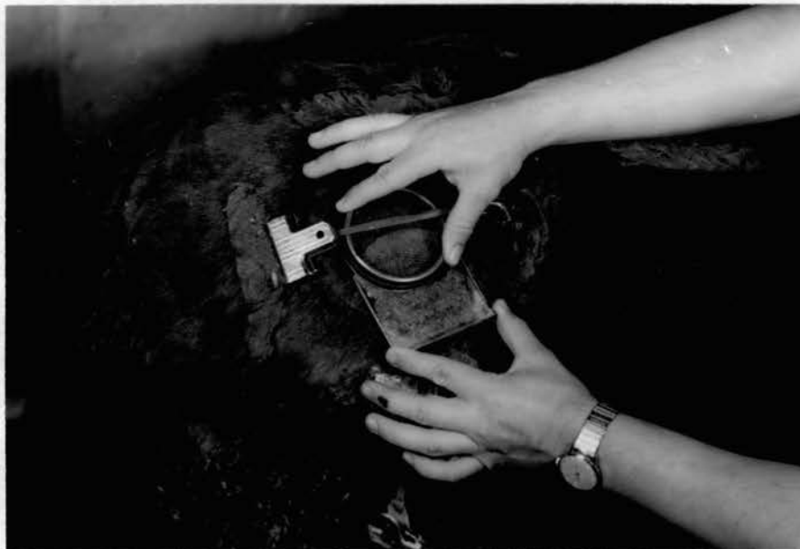
Fig. 10.--Placing the spot test cage in position under one of the bands that hold the cage during exposure.
