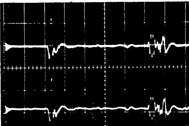
Figure 30b. Fast and Slow Shear Wave Arrivals Propagating Through the Upper Layer of New Rail in the Vertical Plane and at 90^\circ to the Rolling Direction (Specimen T13) Top Trace - 0^\circ Polarization, Bottom Trace - 90^\circ Polarization. Time Base 0.5 \mu\text{s}/\text{div.} )
