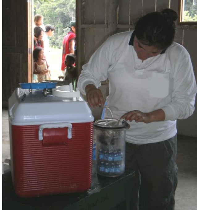
Figure 3. Anaerobic sampling. Picture shows the use of a catalyzer to remove oxygen from chamber. To prevent exposure to oxygen, aliquots were kept in an anoxic airtight container and then placed on ice inside coolers.
