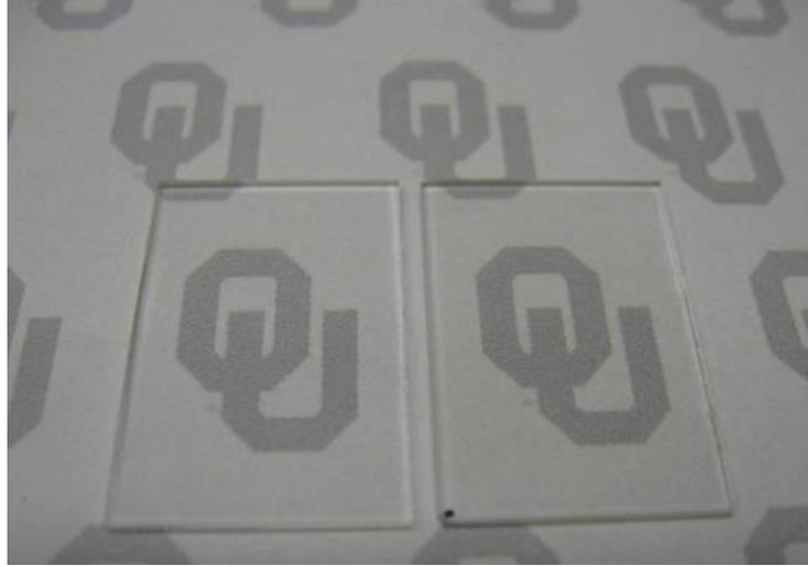
**Figure 46** Optical photo showing quartz substrates without (left) and with a SWCNT film (right). The black dot on the bottom left corner of the right substrate was used as a marker for the side with the film.
