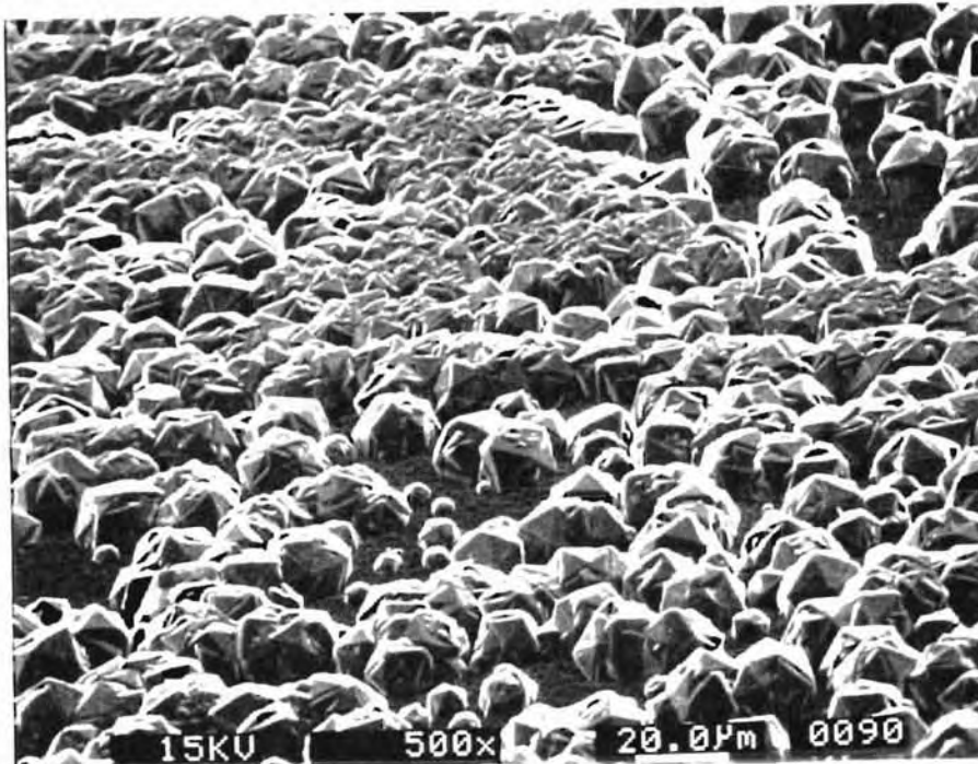
Figure 7.6.2.4 b) SEM Micrograph Showing Island of Cubo-Octahedral Diamond Crystals on WC621
