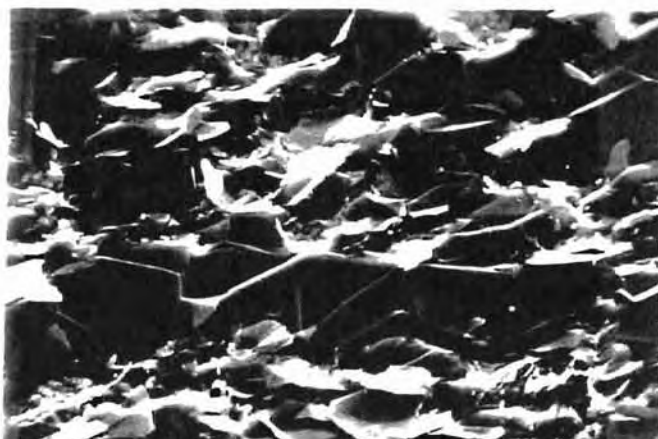
Figure 8.3.3 f) SEM Micrograph of the Co Substrate after Removing the Diamond Film that has been Peeled off Showing Flaky Graphite
