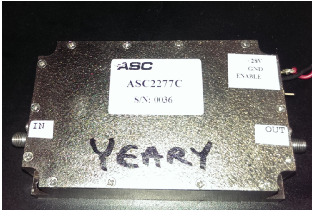
Figure 6.3: High Power Amplifier
