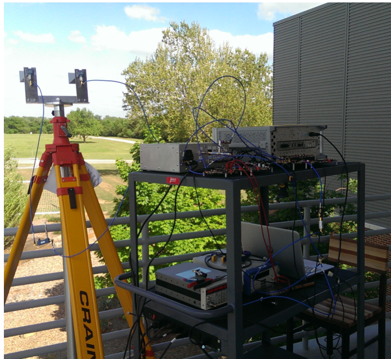
Figure 8.6: System Used for Range Doppler Measurements
