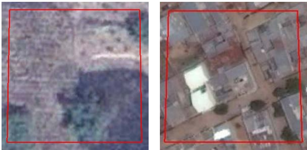
Figure 3.4. Two data points (30 m × 30 m) collected using the Google Earth™. The pixel on the left panel shows a mix land cover classes, cropland (70%) and grass and herbaceous near Abuja, Nigeria. The pixel on the right panel shows a mixed pixel with buildings (80%) and unpaved roads (20 %) near Kano, Nigeria.
