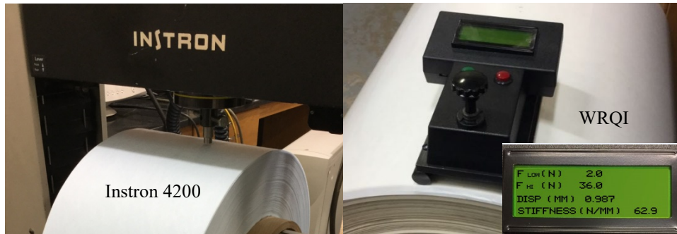
Figure 3 – Surface Stiffness Testing Instruments: Instron 4200 and WRQI
