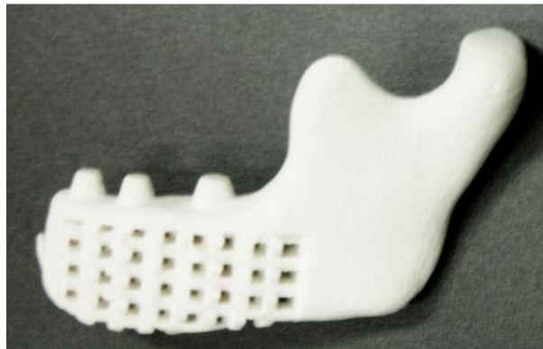
Figure 4. 22 3DP model of porous mandible
