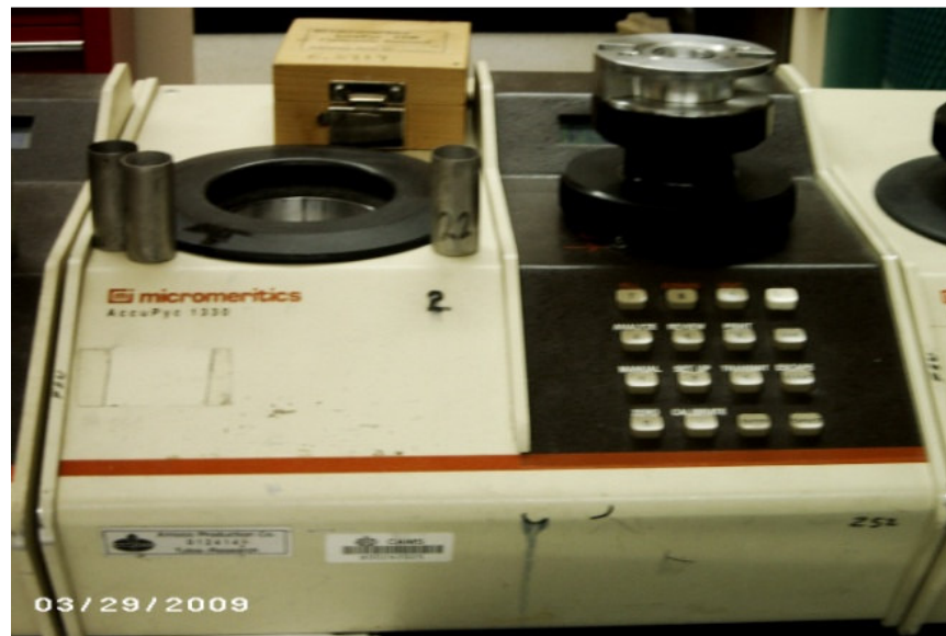
Figure 5. 8 Helium gas Pycnometer used for estimation of pore volume
