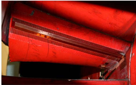
Figure 2.10: Plasma actuator on a compressor blade: approx.  $1/4$  chord
