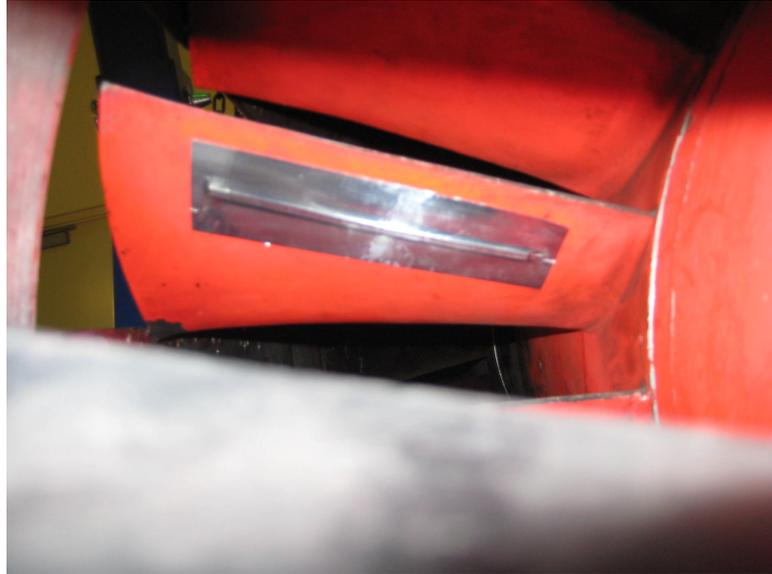
Figure 3.11: Mechanical trip installed at 1/4 chord
