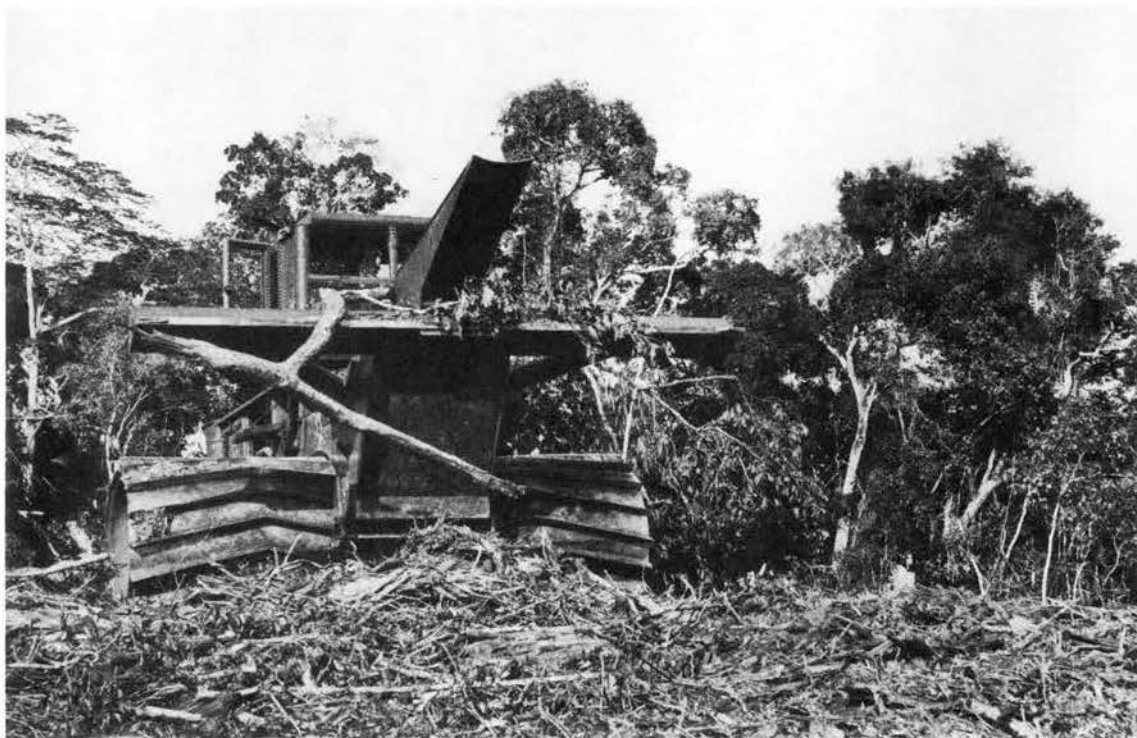
Figure 56. "Business-end" of LeTourneau Tree Crusher, Results in Foreground
