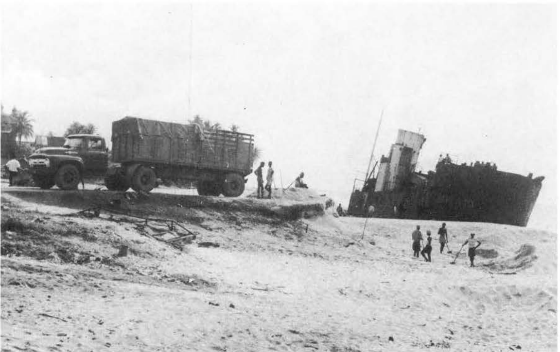
Figure 21. M/V Robert G. Hopelessly Mired in 8 Feet of Sand After Drifting Cross-wise on Beach
