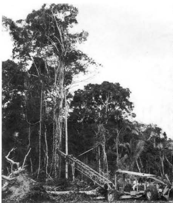
Figure 41. LeTourneau "Tree Stinger" Pushes Over a Big One Bypassed by the Bulldozer
