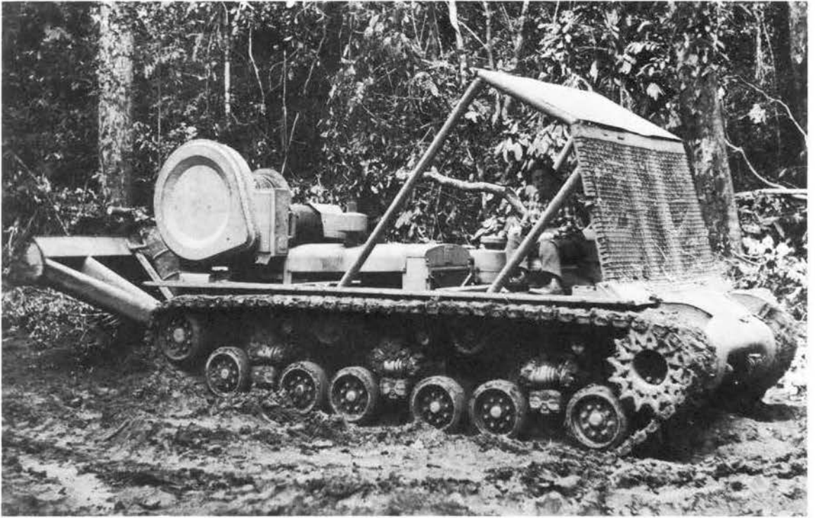
Figure 22. Surplus Army Tank With Converted Electric Drive Utilized as a Bulldozer During Road Contract
