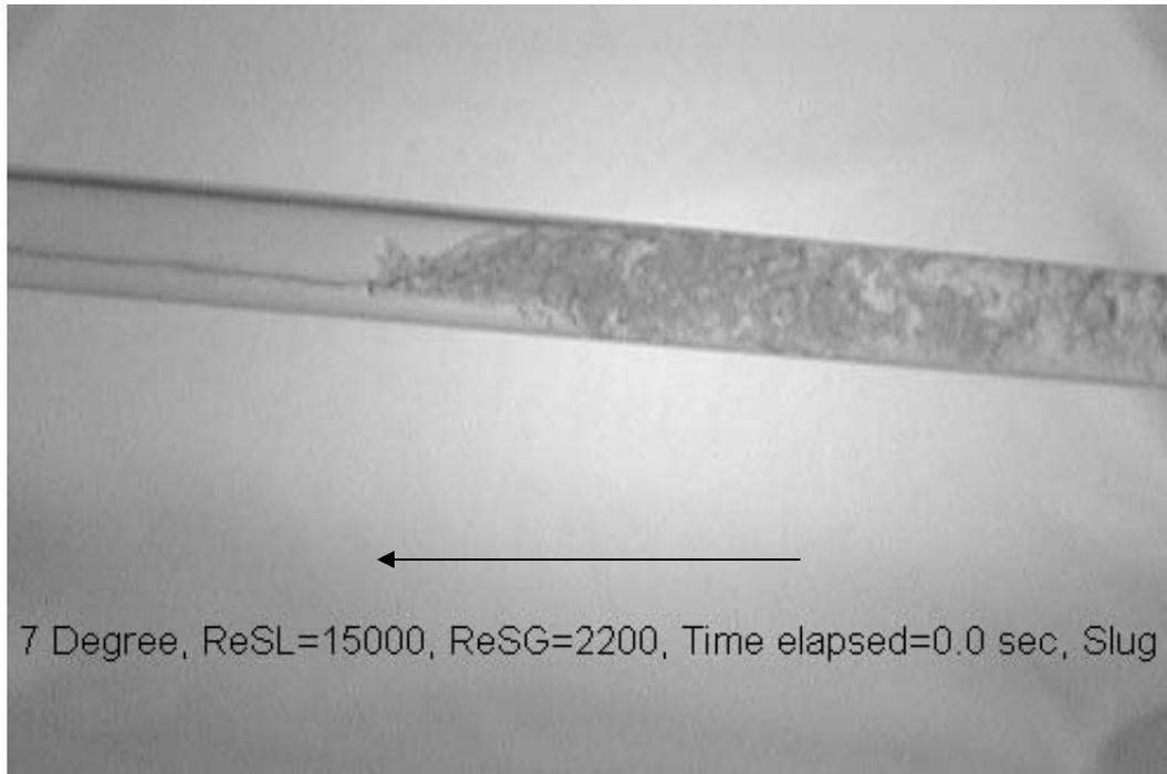
Figure 4.49 (b) – Seven degree slug flow at time 0.0 sec ( $Re_{SL}=15000$ ,  $Re_{SG}=2200$ )
