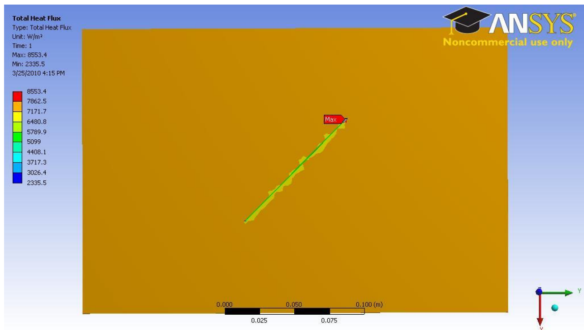
Fig. 4.2 Image of Temperature Gradient Resulting from an Angled Crack from ANSYS Model.
