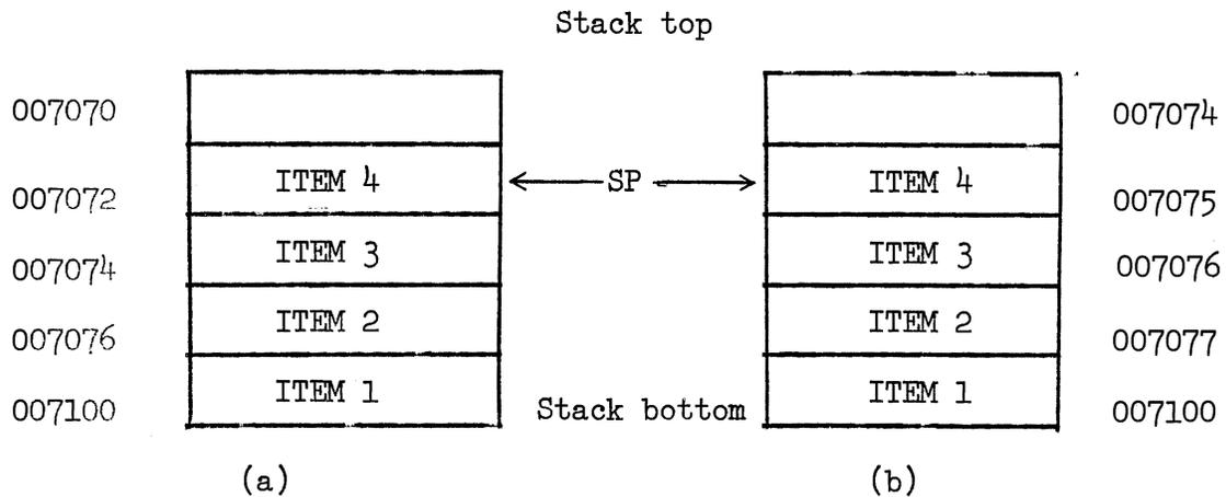
Figure 7. Processor Stacks (a) Word Stack (b) Byte Stack
