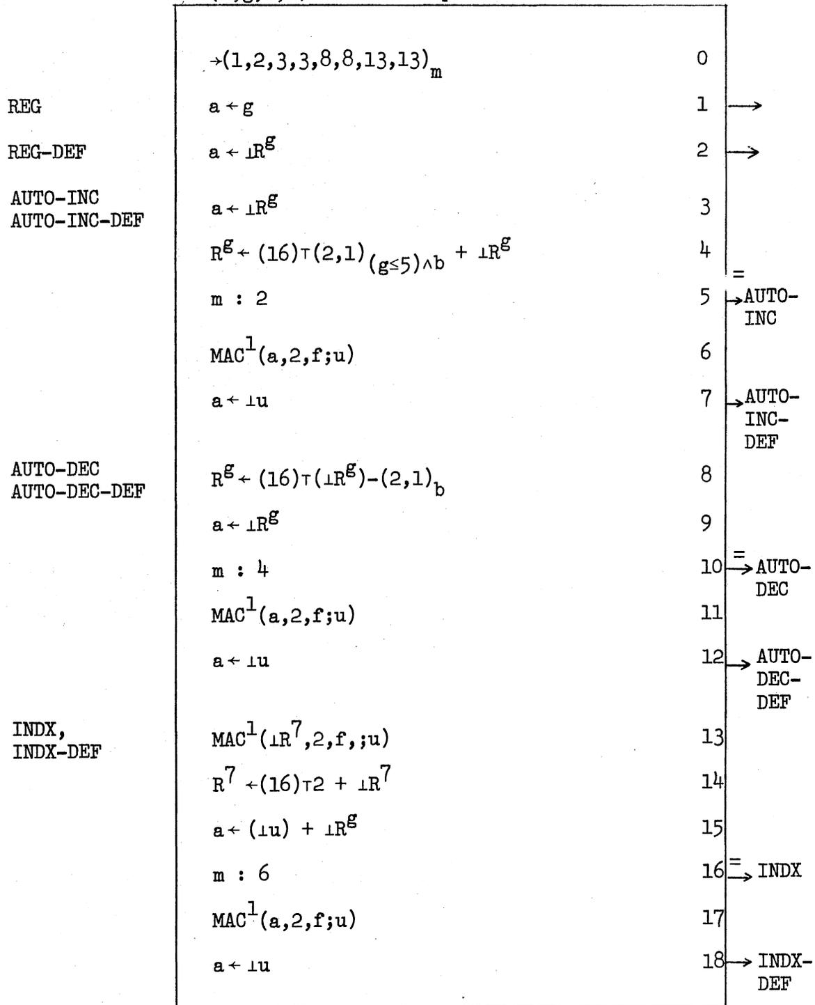
Figure 23. Address Computation Operation
