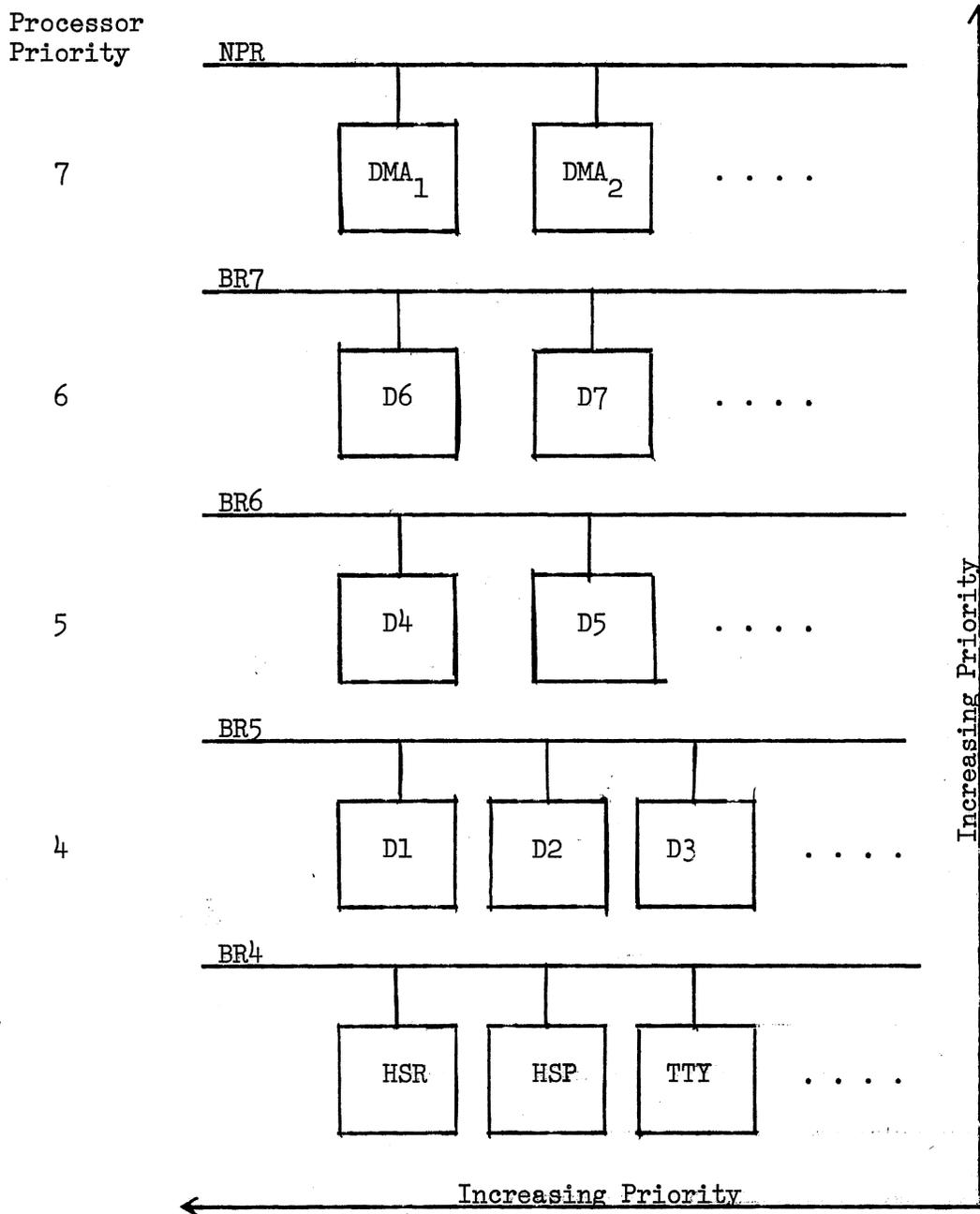
Figure 8. Priority Interrupt Structure (11)
