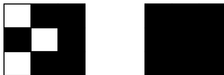
Figure-7: Superimposition of white and black subpixels
