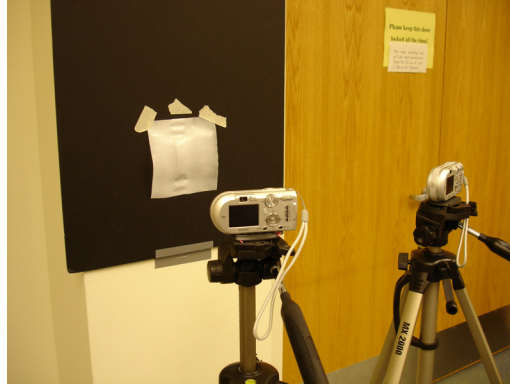
Figure 5.10 : Experimental setup used for the polyethylene web with real baggy lanes.
