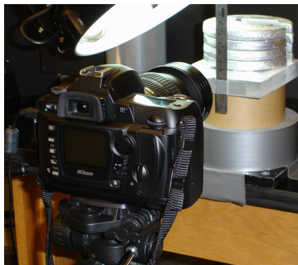
Figure 3.18 : Experimental setup used for observation of out-of-plane viscoelastic recovery.
