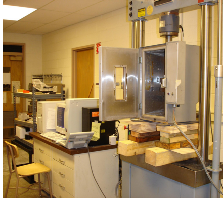
Figure 4.16 : The experimental setup used to conduct out-of-plane viscoelastic material property characterization.
