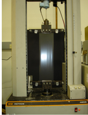
Figure 3.24 : Experimental setup used to determine the critical buckling load during the onset of wrinkling.
