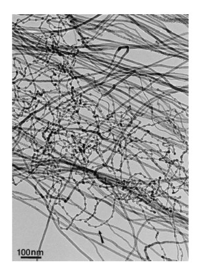
Figure 2.15 TEM image showing two major morphologies of Si nanowires (113).
