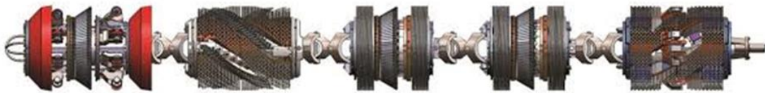
Figure 4: A Multi-Data Set (MDS) tool used during pipeline inspection to check for pipeline anomalies. This MDS tool utilizes multiple scanning techniques such as MFL, IMU, geometry, and ID/OD modules. Courtesy of T.D. Williamson.
