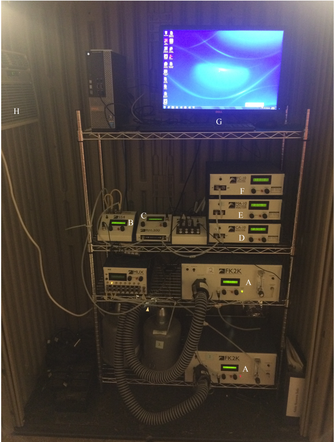
Figure 7. The instrumentation cabinet containing the FlowKits (A), SS-4 sub-sampler pump (B), RH-300 water vapor analyzer (C), CA-10 carbon dioxide analyzer (D), MA-10 methane analyzer (E), FC-10 oxygen analyzer (F), computer (G), and A/C unit (H) located adjacent to the head boxes.
